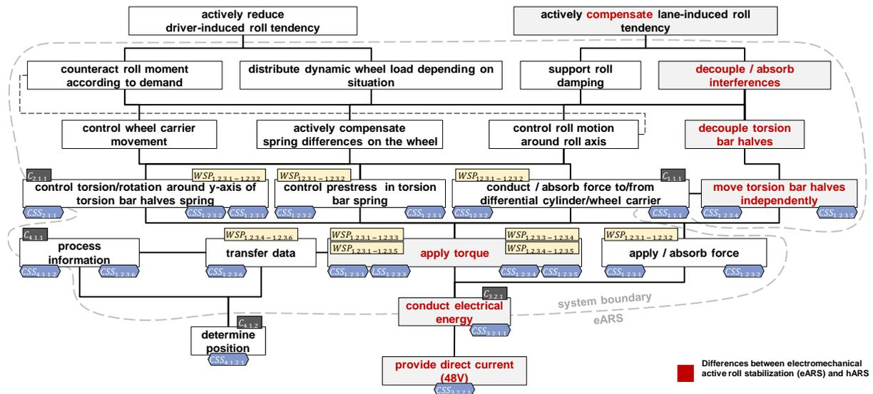
Figure 20: Function structure of the electromechanical active roll stabilization system (eARS) compared with hARS
