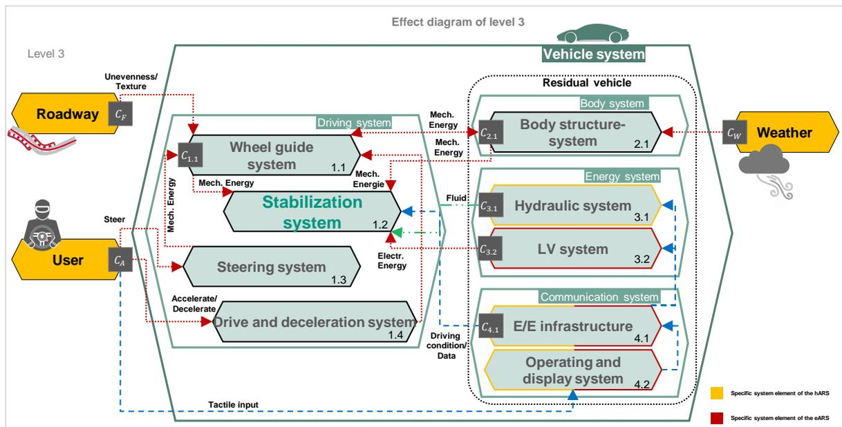
Figure 12: Effect diagram of level 3: Stabilization System
