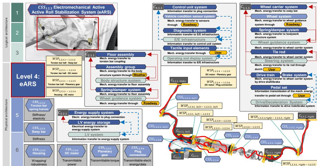
Figure 19: C&C<sup>2</sup> model on level 4: Electromechanical Active Roll stabilization (eARS)<sup>8</sup>
