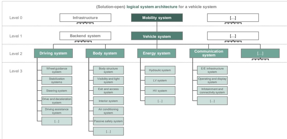
Figure 8: Excerpt of the used (*solution-open*) logical system architecture for a vehicle system in the study
