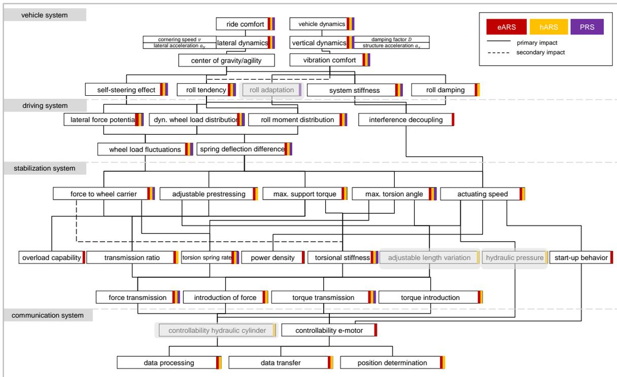
Figure 21: Property structure of the electromechanical active roll stabilization system (eARS) compared with hARS
