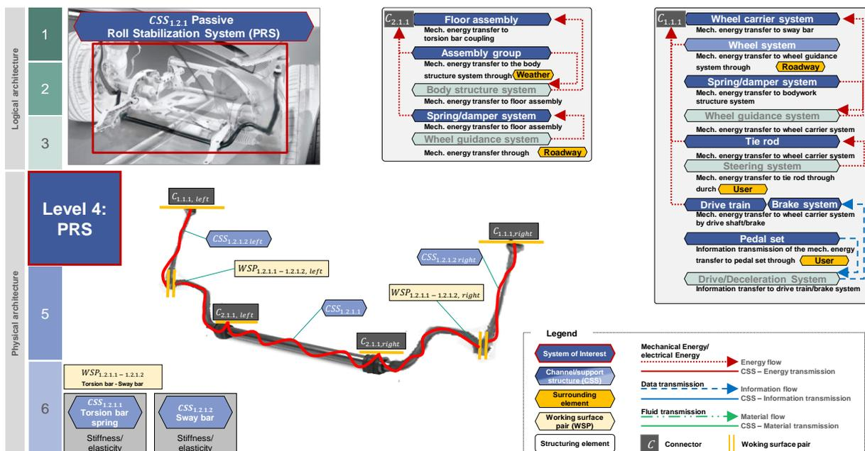
Figure 13: C&C<sup>2</sup> model on level 4: Passive Roll stabilization (PRS)<sup>6</sup>
