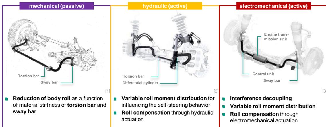
Figure 5: Overview of the alternative reference system elements (RSE) considered for passive, hydraulic active and electromechanical active roll stabilization<sup>3</sup>
