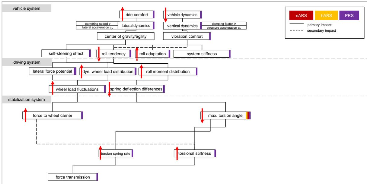
Figure 15: Property structure of the passive roll stabilization system (PRS)
