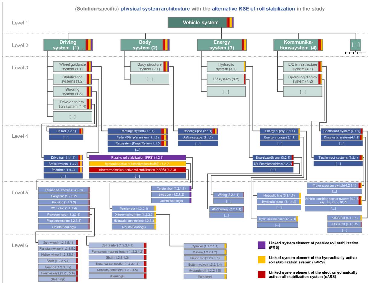
Figure 9: Excerpt of the used (solution-specific) physical system architecture for levels 4,5 and 6 in the study
