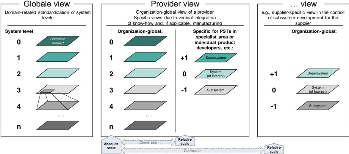
Figure 7: Understanding of system levels in the model of PGE
