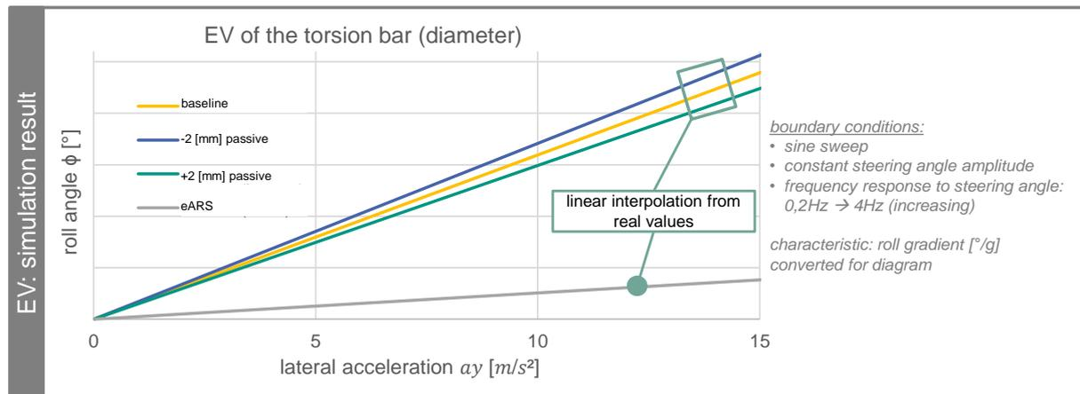
Figure 26: Simulation result in relation to the effects of an embodiment variation
