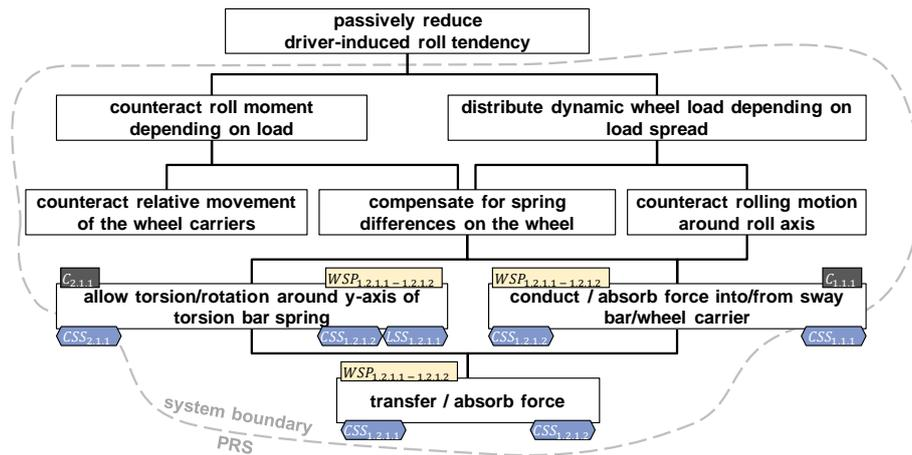
Figure 14: Function structure of the passive roll stabilization system (PRS)
