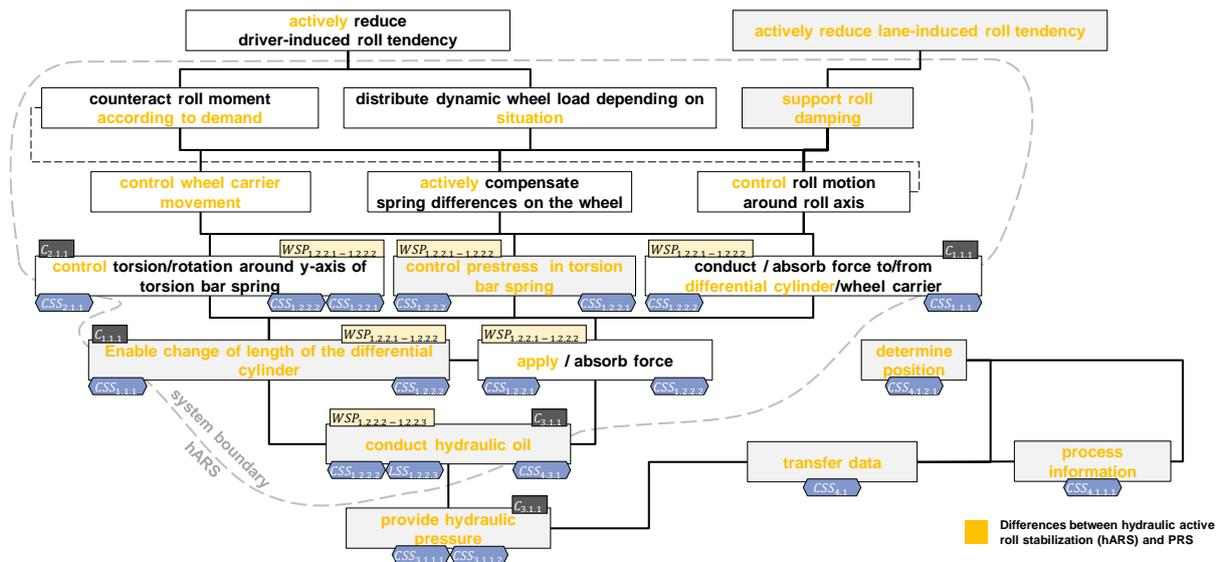
Figure 17: Function structure of the hydraulic active roll stabilization system (hARS) compared with the PRS
