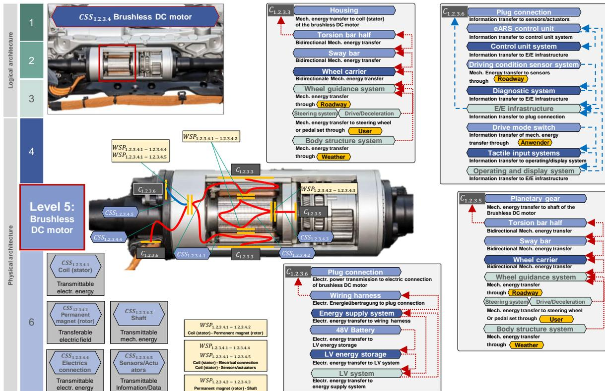
Figure 22: Selected example of a C&C<sup>2</sup> model on level 5: eARS brushless DC motor<sup>9</sup>
