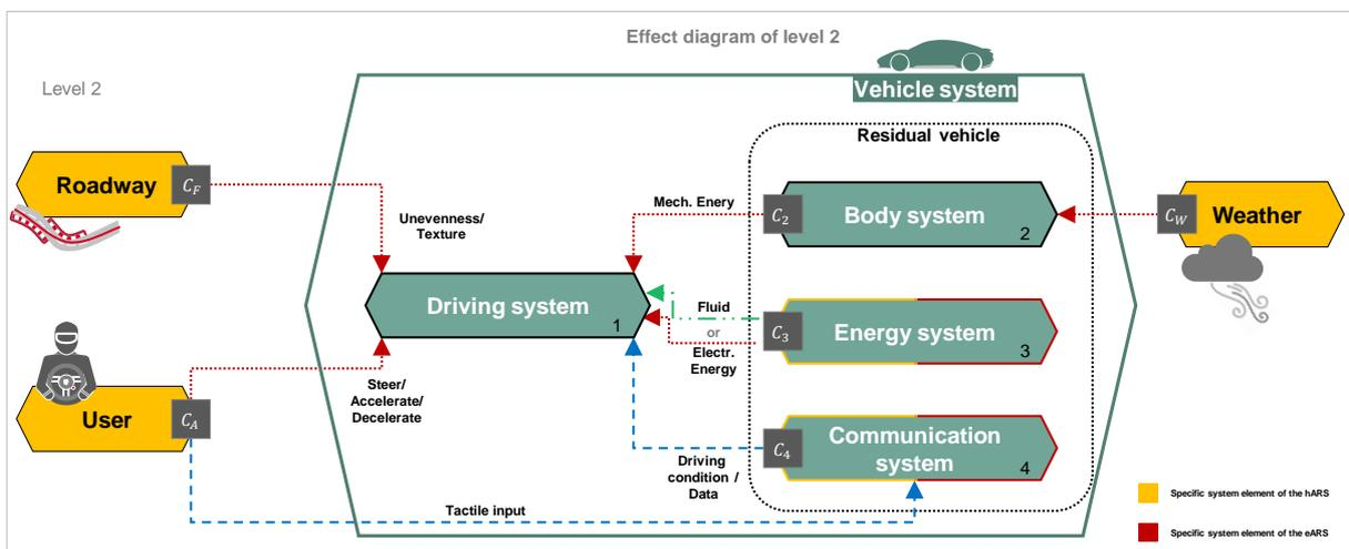
Figure 11: Effect diagram of level 2: Driving System
