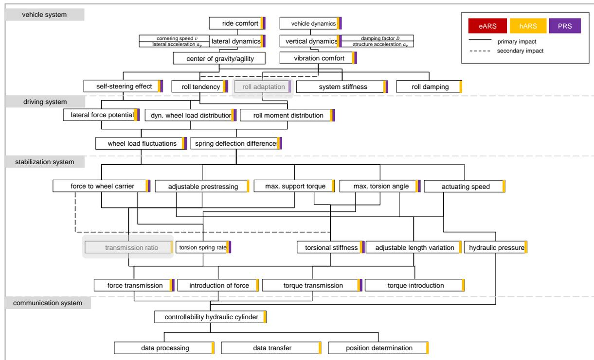
Figure 18: Property structure of the hydraulic active roll stabilization system (hARS) compared with the PRS
