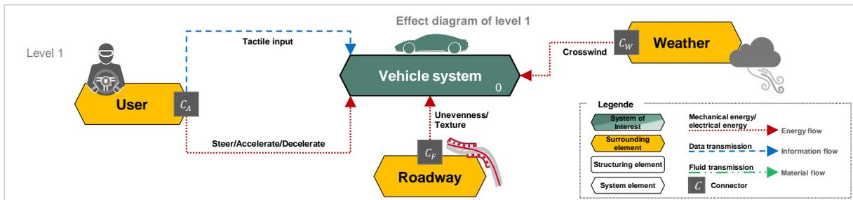
Figure 10: Effect diagram of level 1: Vehicle System
