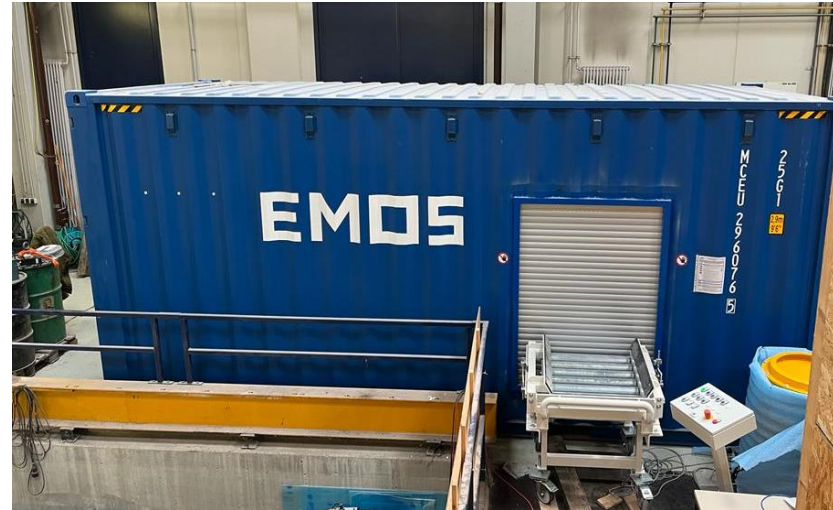
20ft high cube container with a rolling gate at the long side
