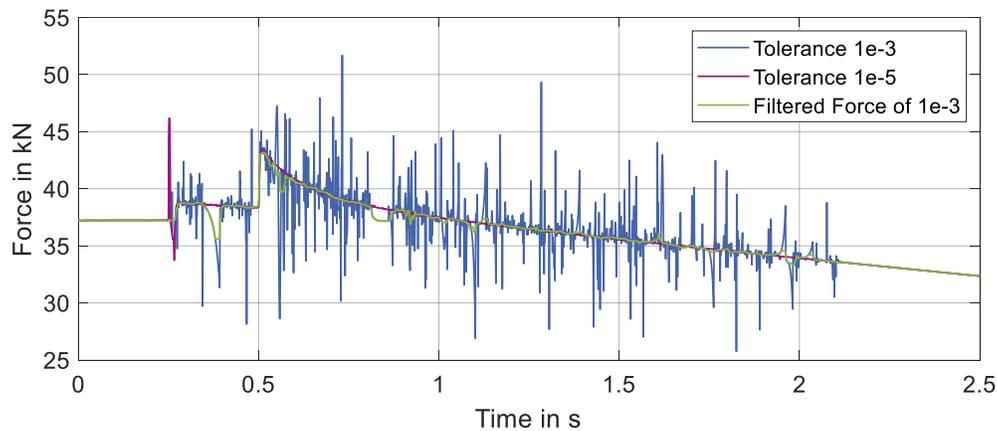
Figure 4. Comparison of simulation result of the vertical ground force over time for two relative error tolerances of the solver and a filtered output.
