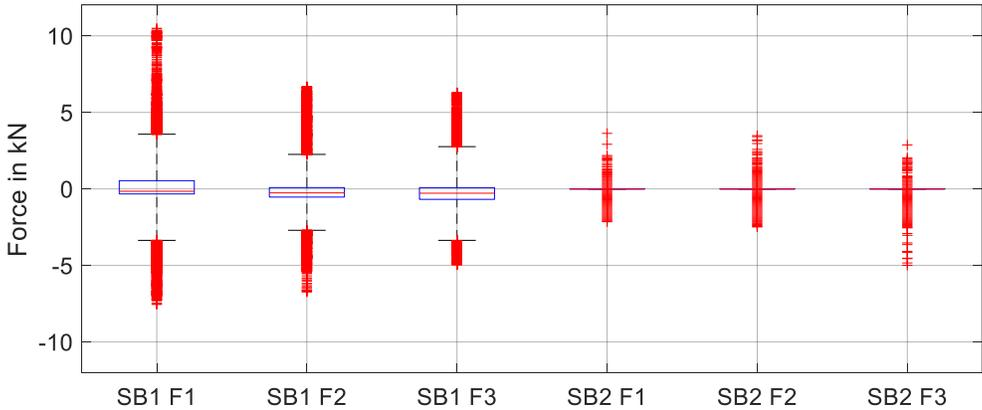
Figure 6. Difference between the calculated and filtered ground force for each foot.
