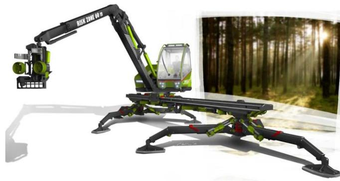
Figure 1. Representation of the portal advancing mechanism with a harvester crane. (Knobloch, 2017)
