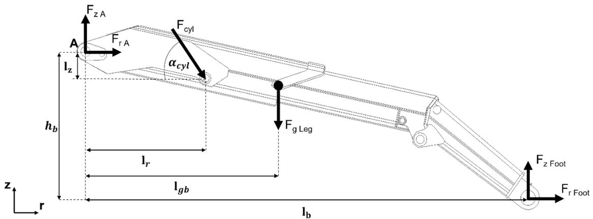
Figure 3. Free cut of one leg of the portal advancing mechanism
