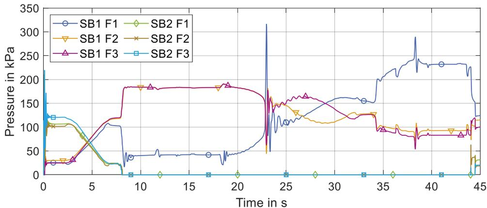
Figure 7. Introduced soil contact pressures of the legs of the portal advancing mechanism during one entire movement cycle calculated with the pressures in the hydraulic system.
