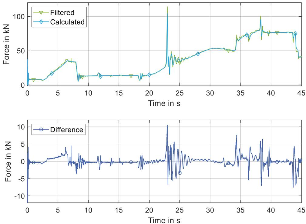
Figure 5. Comparison between the filtered and calculated ground force for the leg with the highest load their difference
