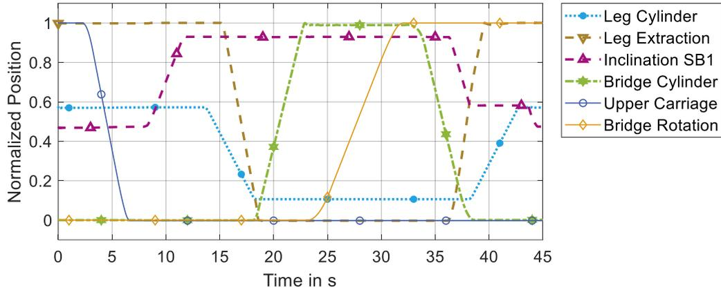
Figure 2. Relative positions of the actuators through one movement cycle.
