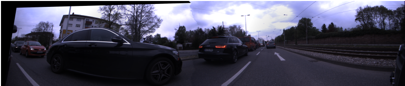
(b) Image stitching with vignetting compensation but without exposure correction.
