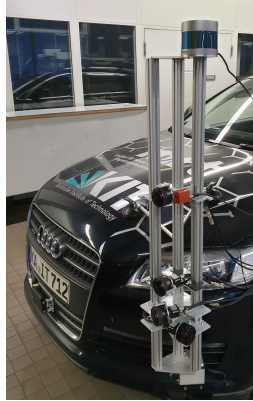
(a) Sensor setup prototype for UNICARagil project.
