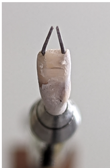
Figure 3.4: Image of an exemplary custom-built hot-wire probe.
