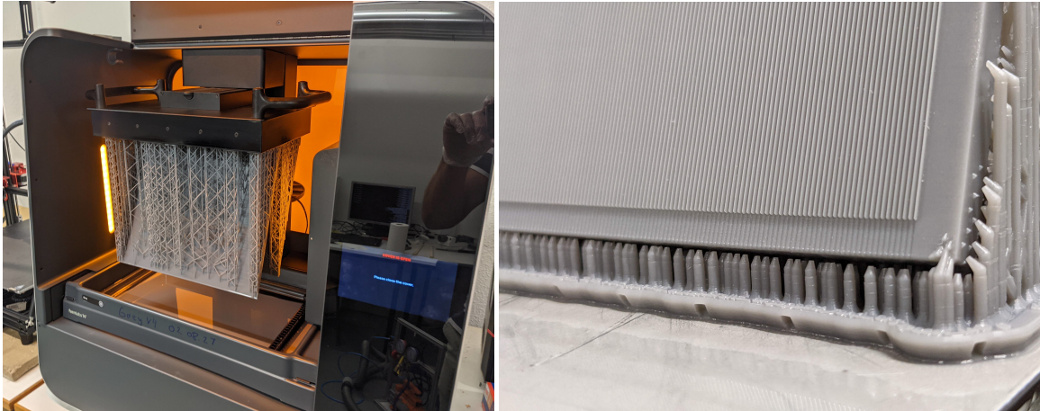
Figure B.6: 3D printed parabolic riblets. (a): completed print of two riblet plates. (b): Detailed view of the 3D printed riblets, including the support structure employed in the printing process.
