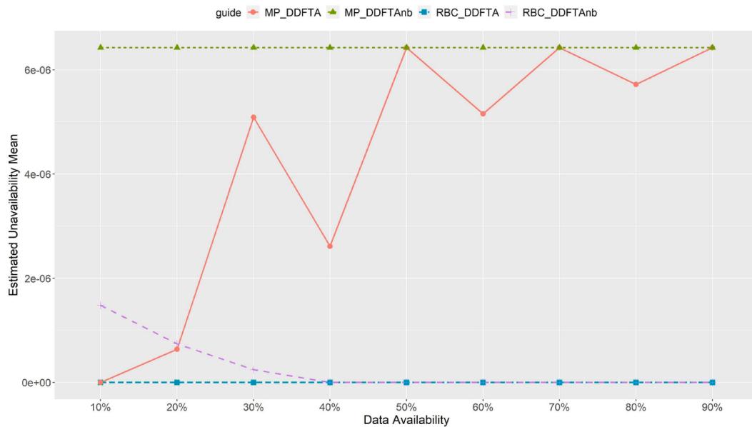
Fig. 15. \hat{U}_n means of MP and RBC fault trees, considering different levels of data availability, for DDFTA and DDFTAnb.
