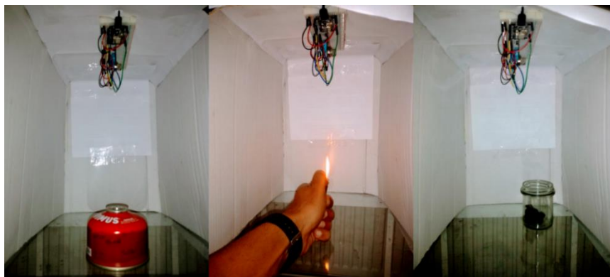
Figure 7. Gas leak (left), fire incident (middle), and smoke (right) simulation.
