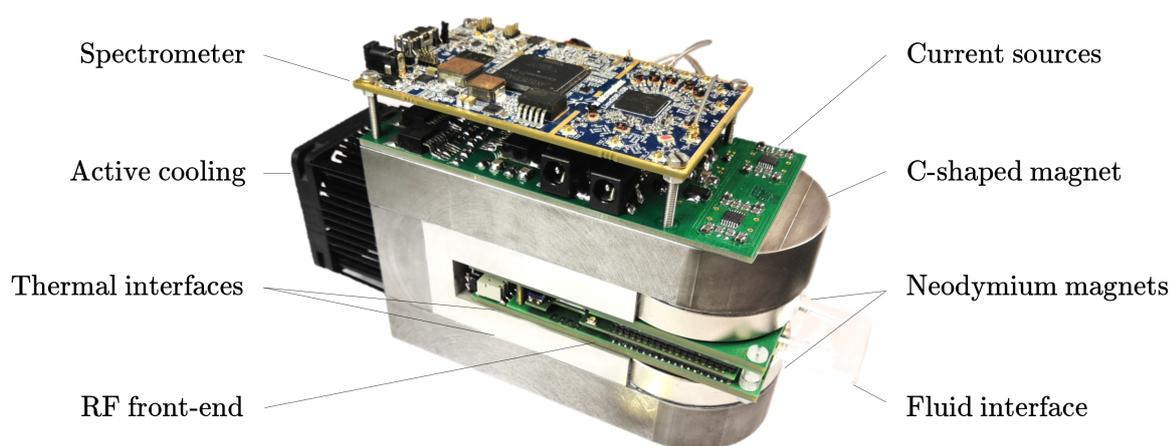
**Figure 3.1:** Photograph of the assembly of the complete prototype fabricated. Picture includes the front-end for NMR signal transception, a LimeSDR spectrometer with a USB connection, a bi-planar set of shims/gradients, a board containing controllable current sources and a C-shaped gap magnet with a thermal management system. A disposable PMMA planar insert, containing the flowing sample, is shown entering the user-accessible front of the setup, on the right.
