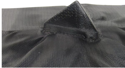
Figure 2.10: Photograph of large scale textile wrinkling after forming [36]
