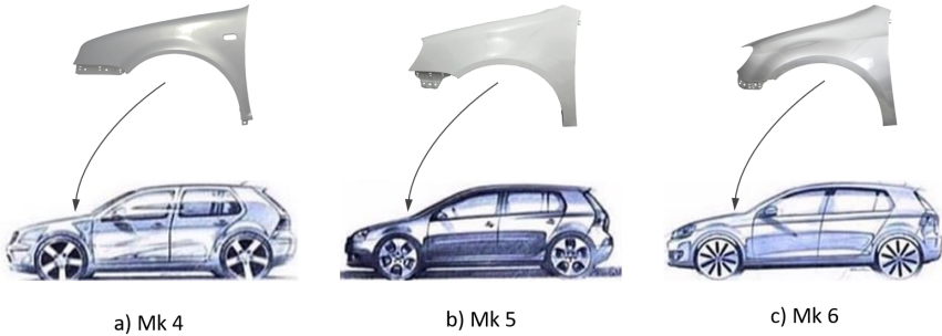
Figure 2.4: Recurring component characteristics during design revisions at the example of the VOLKSWAGEN GOLF's front mudguard (Mk4-6). While the mudguard retains its overall engineering design it varies slightly in shape. Images from [11, 12].
