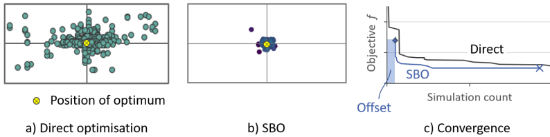
Figure 2.20: History of candidate solutions during a) direct optimisation with a genetic algorithm (GA) and b) SBO. Sub-figure c) shows a faster reduction of the objective f (convergence) over the iterations for SBO [180, 181].
