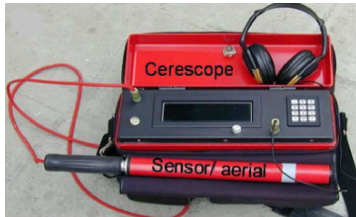
FIGURE 3.18: The Cerescope measuring unit with an aerial sensor and headphones (Greiling and Obermeyer 2010).
