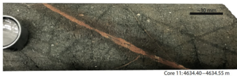
FIGURE 3.13: A piece of core 11 from 4'634.40 to 4'634.55 m depth. It shows felsite veins and conjugate sets of older fractures/veins. The mixture of supercritical vein fluid with cold oxidizing drilling fluid causes the red color of the felsite (Friðleifsson et al. 2017).
