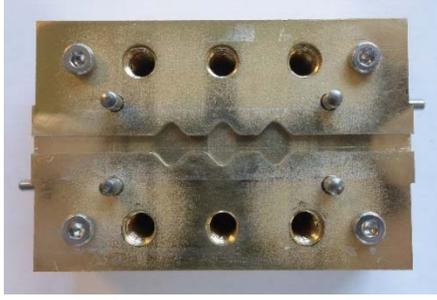
Fig. 7. Three-cavity 105-/140-GHz filter for the F-band, realized in split-block technology.
