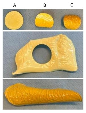
Figure 255: pictures of membranes and their samples: top: A: Top side of a poly(TSC) membrane obtained by using 15wt%polymer solution in DMSO without further treatment. B and C: Poly(TSC) membrane obtained by using a 16wt% polymer solution in DMSO and a 17.9 mM  $AgNO_3$  aqueous solution as non-solvent in the NIPS process. Depicted is the bottom (B) and top side (C). center: Respective membrane of the sample shown in top A. bottom: respective membrane of the sample of top B and C.
