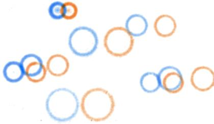
**Figure 5.5:** Random double frame raw image, color-coded and inverted for clarity. blue: frame 1; orange: frame 2. The circle pairs directly indicate larger particle displacements with increasing distance from the focal plane. (Figure adopted from [LFMK21].)
