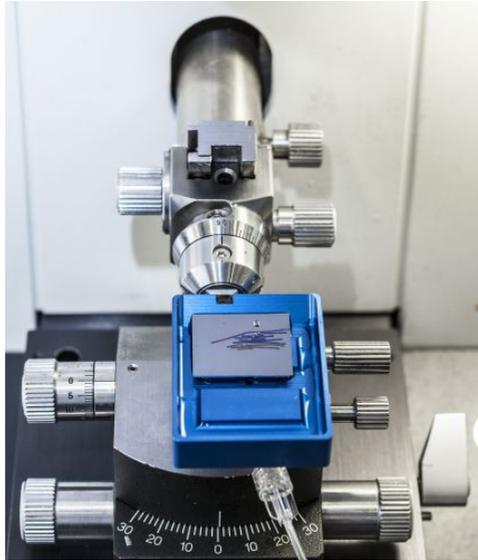
**Figure 2.6:** Diatome ATS knife presented by Burel et al. [45, 46]. The carrier substrate is placed in the bottom of the knife boat. After the section ribbons are positioned above the substrate, the water is drained from the boat using a syringe or valve.
