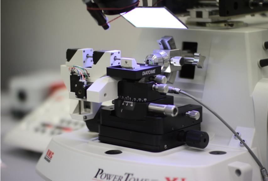
**Figure 4.2:** Integrated system for the machine-based acquisition of serial sections. The edge lit top light is visible overhanging above. The custom black anodized ultra wide knife is mounted on the ultramicrotome. The automated four-axis substrate manipulator is engaged in the knife trough.
