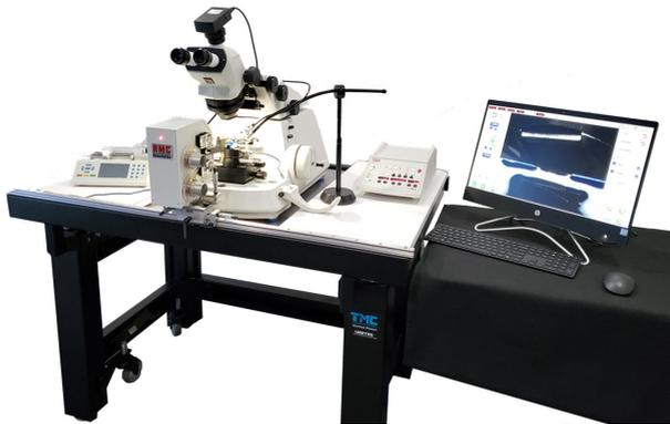
**Figure 2.8:** ATUMtome system to collect serial sections on a flexible tape [29]. The tape collection system is mounted on the front side of the antivibration table and reaches into the knife trough on the ultramicrotome (PT-XL).
