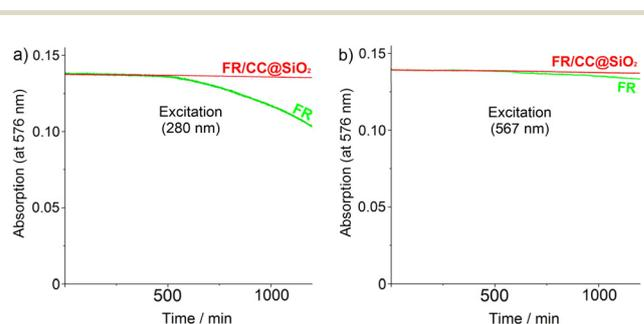
Fig. 6 Photostability of FR/CC@SiO<sub>2</sub> core-shell nanoparticles with continuous exposure for 20 hours at (a) 280 nm, (b) 567 nm (UV-Vis spectra recorded at 567 nm for both types of exposure; aqueous FR/CC@SiO<sub>2</sub> suspension and freely dissolved FR in ethanol with identical FR-load of 2.5  $\mu\text{g mL}^{-1}$ ).
