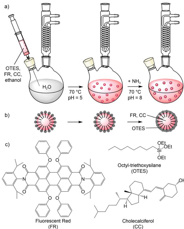
Fig. 1 Schematic illustration of the water-based injection-based synthesis of FR/CC@SiO<sub>2</sub> core-shell nanoparticles: (a) synthesis, (b) structure of nanoparticle, (c) structure of used molecules.
