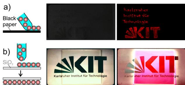
Fig. 8 Thin films with FR/CC@SiO<sub>2</sub> core-shell nanoparticles: (a) scheme of a pen filled with aqueous nanoparticle suspension and photos of written letters without and with excitation ( $\lambda_{\text{exc}} = 366$  nm), (b) scheme of nanoparticles between two quartz-glass plates and photos in daylight and with excitation ( $\lambda_{\text{exc}} = 366$  nm) (due to whitener the paper with the logo shows certain white emission itself).
