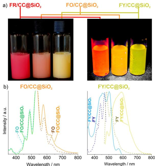
Fig. 7 PD/CC@SiO<sub>2</sub> core-shell nanoparticles with FR, FO, and FY as fluorescent dyes: (a) photos of suspensions in daylight and with excitation ( $\lambda_{\text{exc}} = 366$  nm), (b) excitation and emission spectra (in H<sub>2</sub>O, with emission monitored at  $\lambda_{\text{em}} = 525$  nm/FO, 460 nm/FY and excitation recorded at  $\lambda_{\text{exc}} = 550$  nm/FO, 605 nm/FY).
