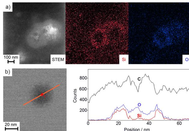
Fig. 3 Structure of FR/CC@SiO<sub>2</sub> core-shell nanoparticles: (a) EDXS area scans with element mapping and (b) EDXS line scan with concentration profile at the position of the orange line on the STEM image.
