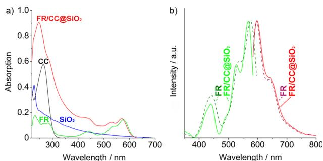
Fig. 5 Optical properties of the as-prepared FR/CC@SiO<sub>2</sub> core-shell nanoparticles (aqueous suspension): (a) UV-Vis spectrum with FR, CC, and SiO<sub>2</sub> as references; (b) excitation and emission spectra with freely dissolved FR as a reference (in ethanol, with emission monitored at  $\lambda_{\text{em}} = 600$  nm and excitation recorded at  $\lambda_{\text{exc}} = 567$  nm).
