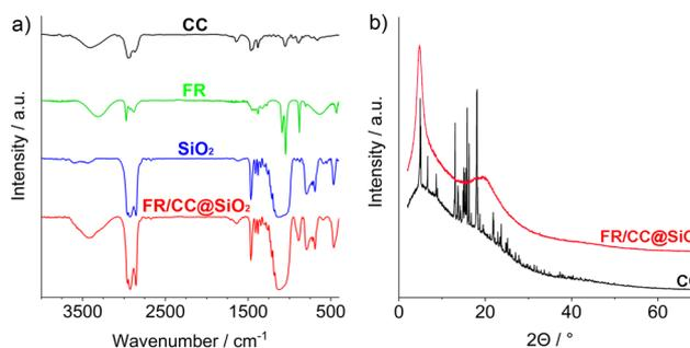
Fig. 4 Chemical composition of the as-prepared PR/CC@SiO<sub>2</sub> core-shell nanoparticles: (a) FT-IR spectra with FR, CC, and SiO<sub>2</sub> as a reference (SiO<sub>2</sub> prepared by hydrolysis of OTES); (b) XRD patterns with CC as a reference.
