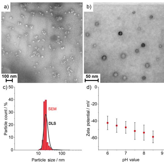
Fig. 2 Size, shape, and colloidal stability of FR/CC@SiO<sub>2</sub> core-shell nanoparticles: (a) particle size according to SEM overview images; (b) particle shape and inner cavity according to STEM detail image; (c) size distribution according to SEM and DLS; (d) zeta-potential of aqueous suspension at different pH values.
