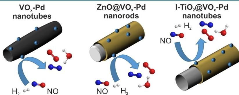
**Nanostructured Catalysts for Selective Reduction of NO:** Vanadium oxide (VO<sub>x</sub>) nanotubes, VO<sub>x</sub>-coated ZnO nanorods, and VO<sub>x</sub>-coated, layered-titania nanotubes are decorated with Pd nanoparticles and
