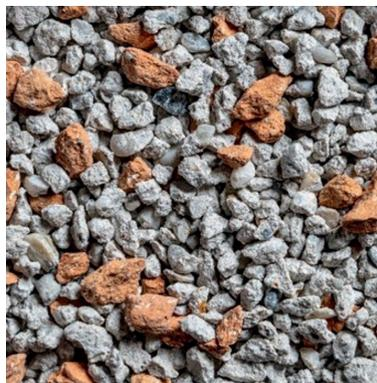
**Figure 1.** Mixture of bulk material to be sorted. Brick (orange) and sand-lime brick (grey).
