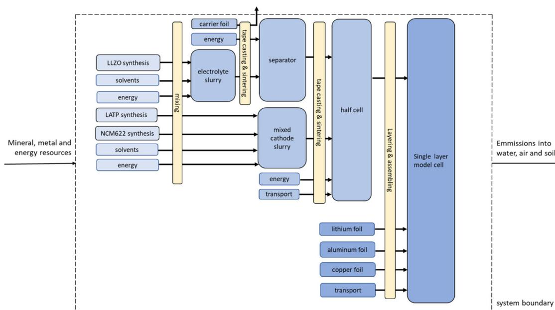
Fig. 3 Flowchart of cell manufacturing adapted and based on ref. 46.
