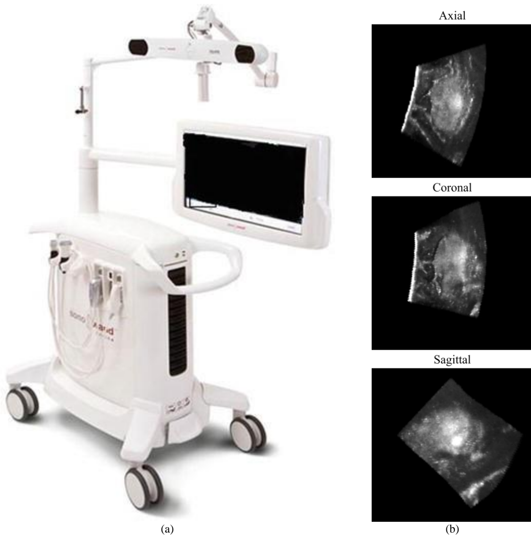
Figure 2.3: An example of a B-mode US scanner (a) and its output images (b) showing the brain tumor which appears in bright grayscale in axial, sagittal, and coronal views (Shetty & Moiyadi, 2016; Xiao, Fortin, Unsgard, Rivaz, & Reinertsen, 2017).
