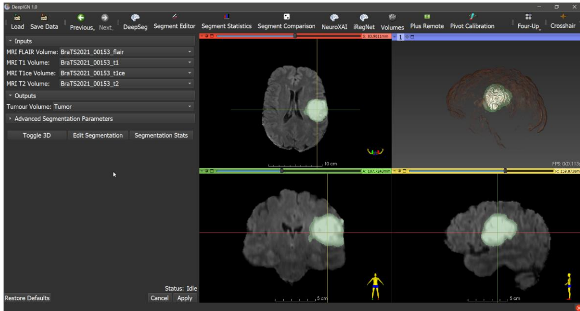
Figure 7.5: DeepSeg module during visualization of the resultant tumor boundaries. The GUI panel is shown on the left, where the user can specify inputs, output volumes, model parameters, and other 3D visualization options. Brain tumor segmentation results ( green ) of a sample HGG case from the BraTS 2021 challenge are presented on the right. The application layout shows the axial ( top middle ), sagittal ( bottom middle ), and coronal ( bottom right ), as well as 3D views ( top right ).
