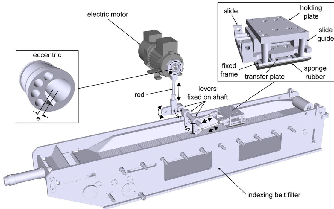
**Figure 3.** Setup to generate oscillatory shear on the indexing HVBF.
