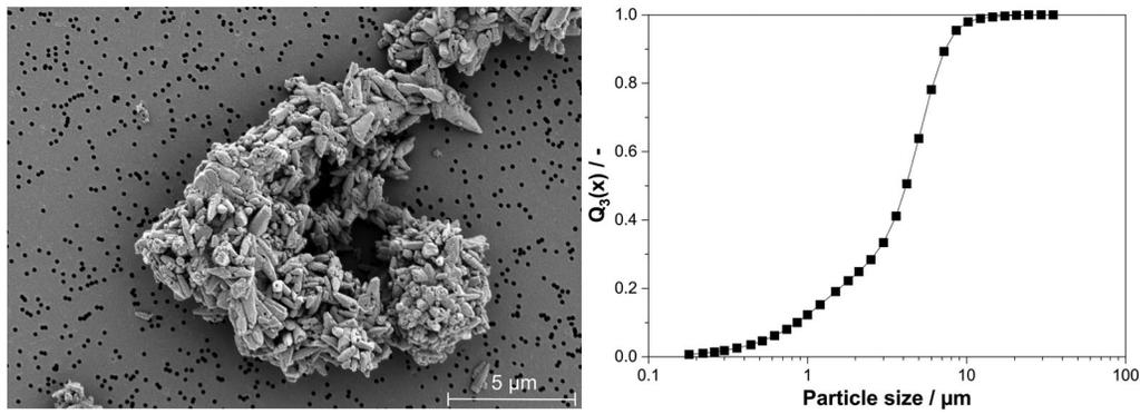
**Figure 1.** Particles of the model material imaged by a scanning electron microscope (left). Particle size distribution of the model material in deionized water, determined by the HELOS H0309 laser diffraction instrument (Sympatec GmbH, Germany) (right).
