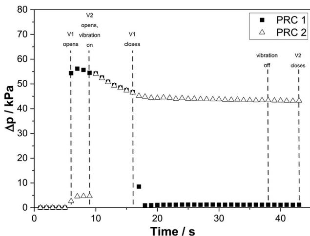
**Figure 5.** Differential pressure in filtrate chambers 1-3 (PRC1) and 4-5 (PRC2) at a cycle time of 43 s.
