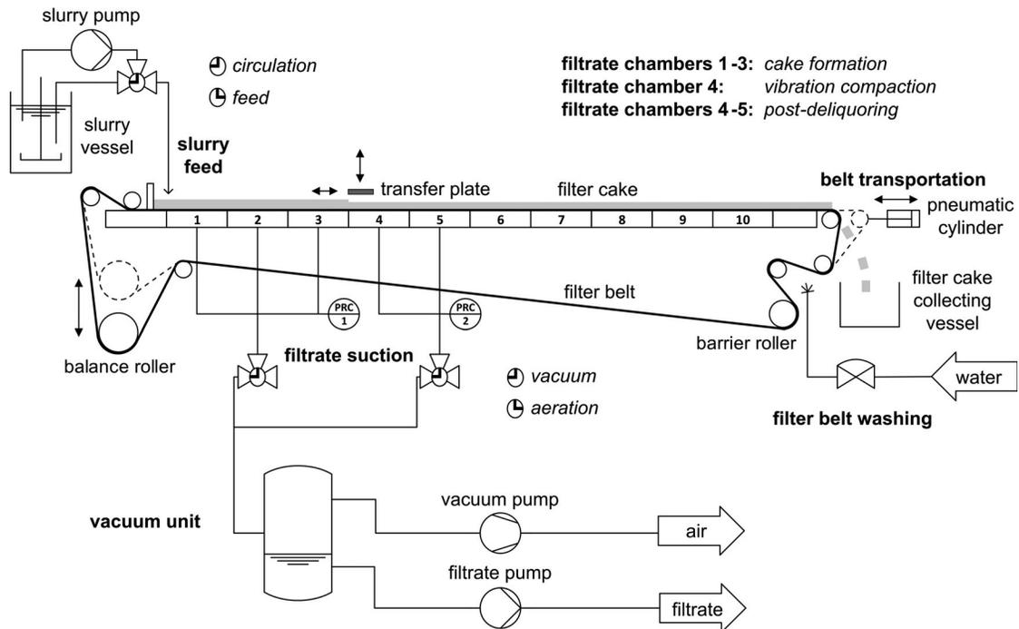
**Figure 2.** Schematic illustration of the indexing HVBF.
