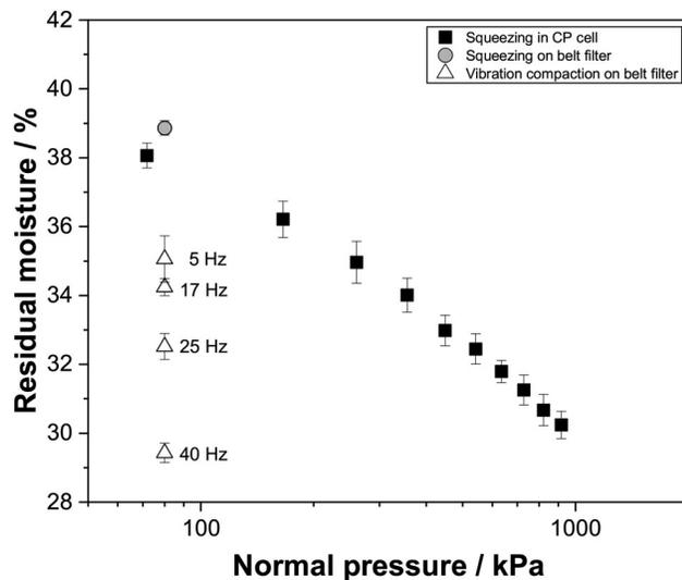
**Figure 11.** Minimum achievable residual moisture of the filter cake after compaction at different normal pressures in the CP cell, after compaction at a normal pressure of 80 kPa, and after vibration compaction at a normal pressure of 80 kPa and a shear length of 4.5 mm on the HVBF. The achievable residual moisture on the HVBF results from data modeling using Eq. 5.
