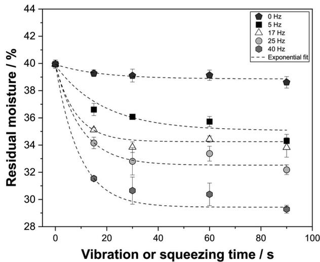
**Figure 8.** Residual moisture of the filter cake after cake formation and after compaction under oscillatory shear at a shear length of 4.5 mm and low normal pressure of 80 kPa on the HVBF. The dashed lines represent the exponential data modeling by using Eq. 5.
