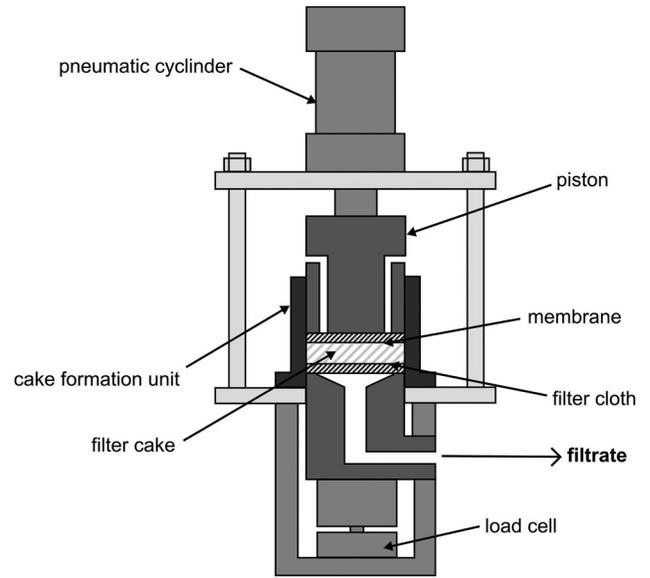
Figure 7. Setup of the CP cell described in detail by Alles.<sup>[30]</sup>
