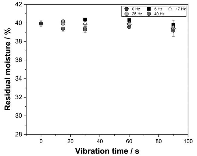
**Figure 9.** Residual moisture after cake formation with and without parallel compaction under oscillatory shear at a shear length of 4.5 mm and low normal pressure of 80 kPa.
