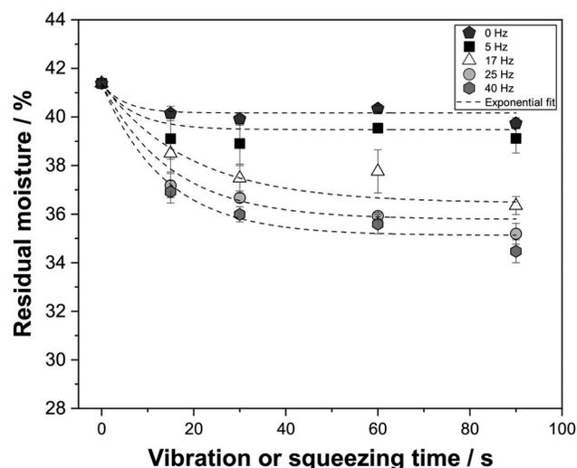
**Figure 10.** Residual moisture of the filter cake after cake formation and after compaction under oscillatory shear at a shear length of 4.5 mm and a normal pressure of 80 kPa in the laboratory apparatus. The dashed line represents exponential data modeling by using Eq. 5.
