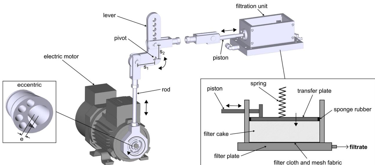
**Figure 6.** Setup of the discontinuous laboratory apparatus developed by Illies et al.<sup>[26]</sup> for the application of oscillatory shear to filter cakes.
