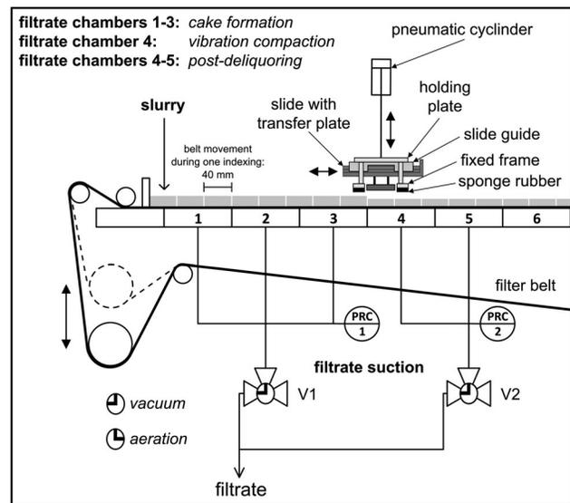
**Figure 4.** Schematic representation of the vibration module installed in the HVBF.
