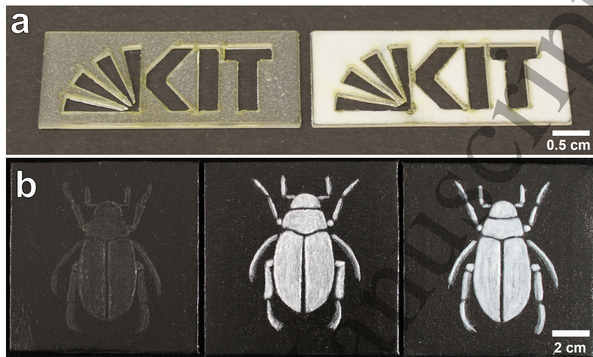
Figure 11. (a) Comparison of a transparent base paint containing either unfoamed (left) or foamed (right) particles at a concentration of 20 wt %, shows a transparent to hazy effect for the mixture with unfoamed particles and a white, opaque coloration for mixtures with foamed particles. (b) The paint containing unfoamed (left), foamed (middle) or PVA-foamed (right) particles can be applied with a brush as well.
