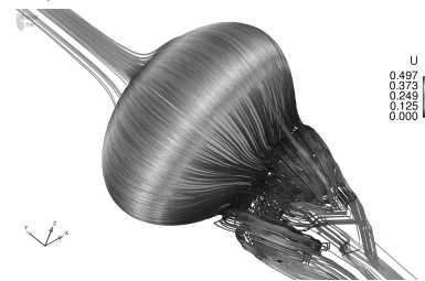
Figure 1 Single rising bubble under the influence of surfactant.
