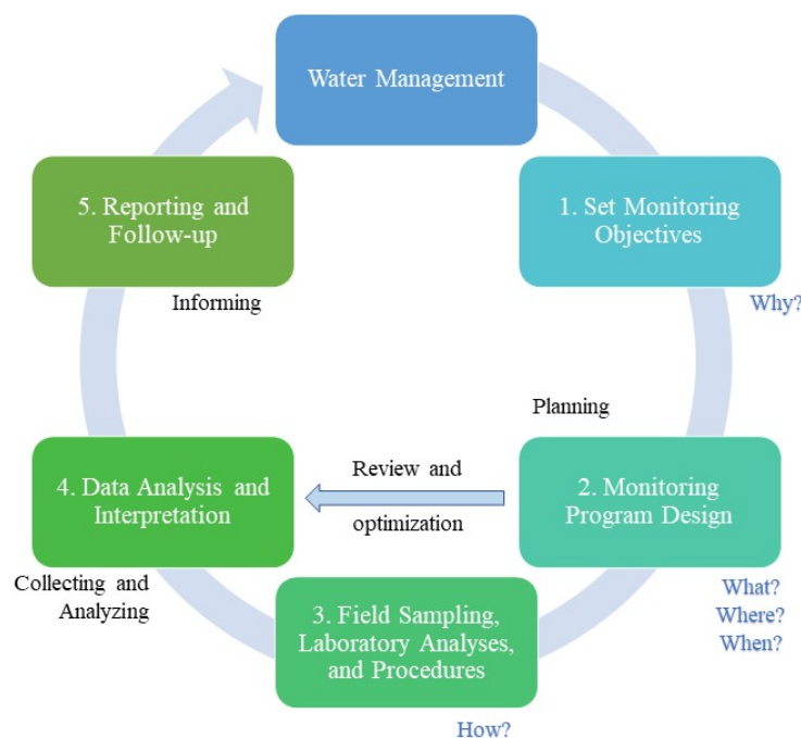
Figure 11 – Summary of different activities, and key processes involved in designing water quality monitoring program
