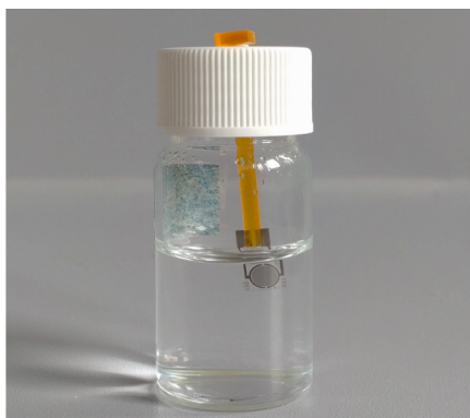
Figure 4.9. Photograph of an IDE chip immersed into a freshly prepared mixture of the ZIF-8 precursor solutions. To avoid the sedimentary deposition of homogeneously nucleated ZIF-8 particles on the surface to be coated, the electrode chip was kept in a vertical position.
