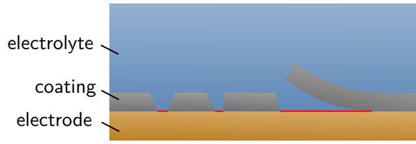
Figure 3.3. Defective coating exposing portions of the bare electrode surface to the reference medium highlighted in red color.
