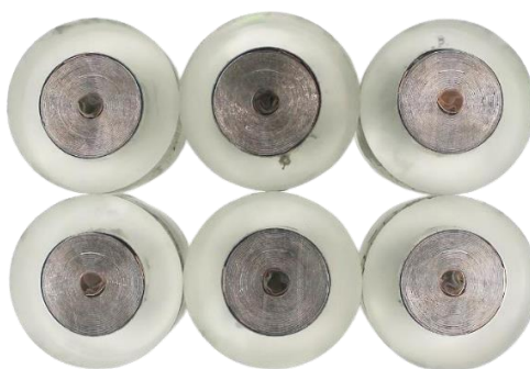
Figure 3-2: Shows cylindrical cross-sections obtained from three cells after the initial grinding step with the SiC abrasive paper.
