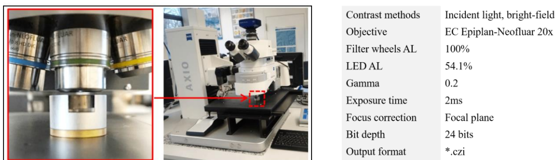
Figure 3-4: Axio Imager.Z2m Vario light microscope (Zeiss) for automated image acquisition of prepared specimen (left). Acquisition parameters for digital imaging of the prepared specimen (right).
