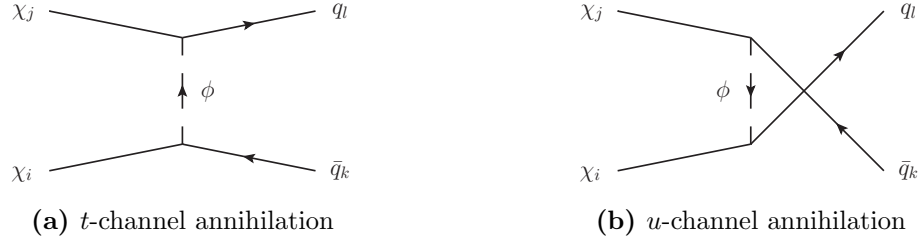
Figure 5.10 | Feynman diagrams for the annihilation of two DM particles into two SM quarks at LO. Note that the u -channel diagram only exists for Majorana fermions.
