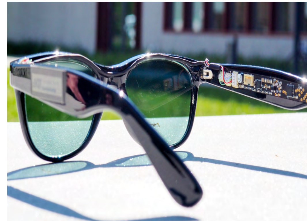
These solar glasses with lens-fitted semitransparent organic solar cells supply two sensors and electronics in the temples with electric power.
