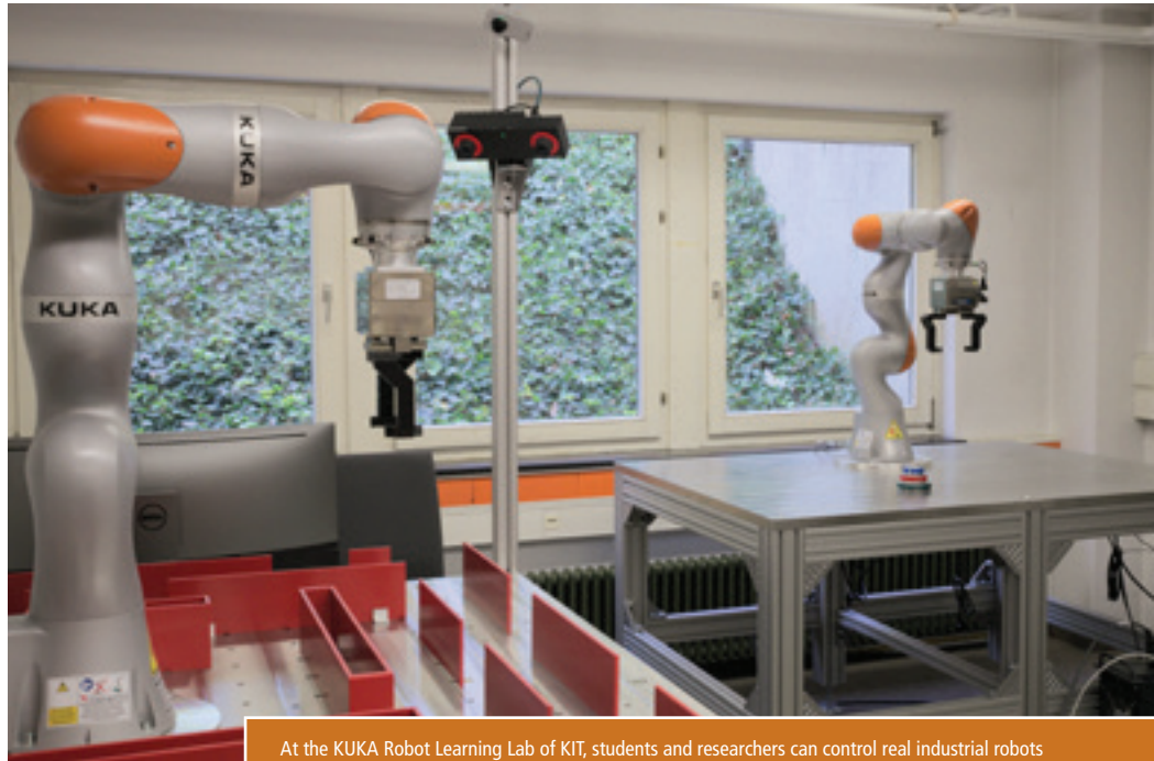
At the KUKA Robot Learning Lab of KIT, students and researchers can control real industrial robots via the Internet and test their routines.
