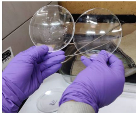
Glass plates spiked with beryllium-containing solution in known amounts were used in the previous study [6]
