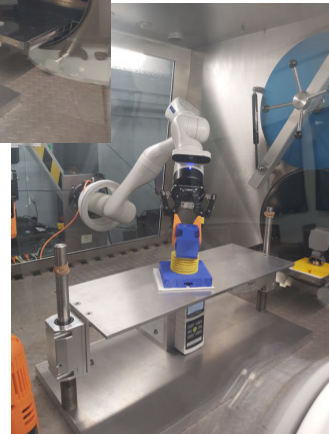
Pressure rig (test fixture) with force gauge installed taking readings from robotic wiping.
