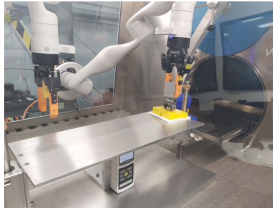
Pressure rig (test fixture) with force gauge installed taking readings from robotic wiping.
