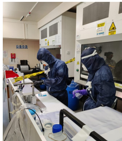
Technicians prepare standardised beryllium samples in a temporary controlled area set up in the Analytical Laboratory at UKAEA expressly for the purposes of this study
