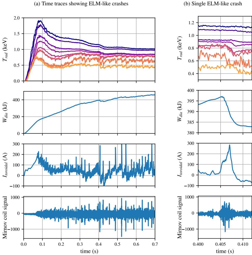
Figure 1: (a) Time traces of the ECE radiation temperature,  $T_{rad}$ , at high field side (HFS) frequencies, the diamagnetic energy,  $W_{dia}$ , the toroidal current,  $I_{toroidal}$ , and the magnetic fluctuations measured by Mirnov coils are shown for the plasma discharge #20180927.026 where the 5/5 island chain was moved inside the last closed flux surface. (b) Zoomed in time traces of (a) at 0.4 s showing the temporal evolution of different parameter during a single ELM-like crash.
