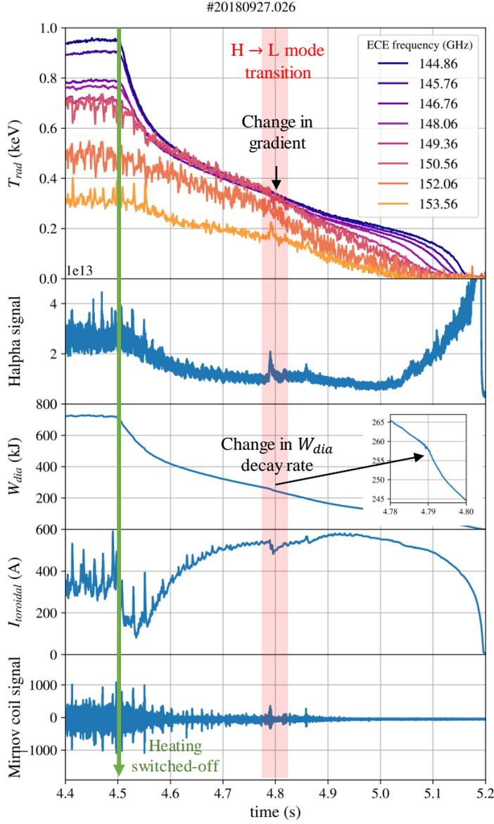
Figure 5: Time traces of ECE, H-alpha,  $W_{dia}$ ,  $I_{tor}$ , and magnetic fluctuations are shown for the plasma discharge #20180927.026 where the magnetic island chain was moved inside the edge confinement region. Plasma heating was switched-off at 4.5 s, and at approximately 4.8 s, transition to a degraded confinement state can be observed through increased  $W_{dia}$  decay rate and changed temperature gradient with occurrence of an ELM-like crash (top plot).
