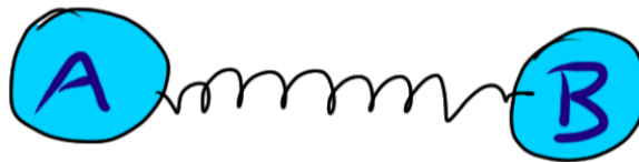
Fig. 1. The spring is under tensional stress. The momentum of A increases, that of B decreases (the “negative momentum” of B increases).
