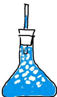
Fig. 1. The amount of entropy that is to be measured is transferred to the ice-water mixture. The amount of the melting ice is a measure of the entropy that has been supplied.
