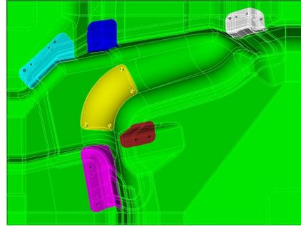
Figure 2: Computer-aided designed experimental die (top view). Insertion element 1 is marked in yellow, 2 in magenta, 3 in light blue, 4 in dark blue, 5 in grey and 6 in dark red.
