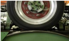
**Fig. 2** Tire rolling on outer drum
