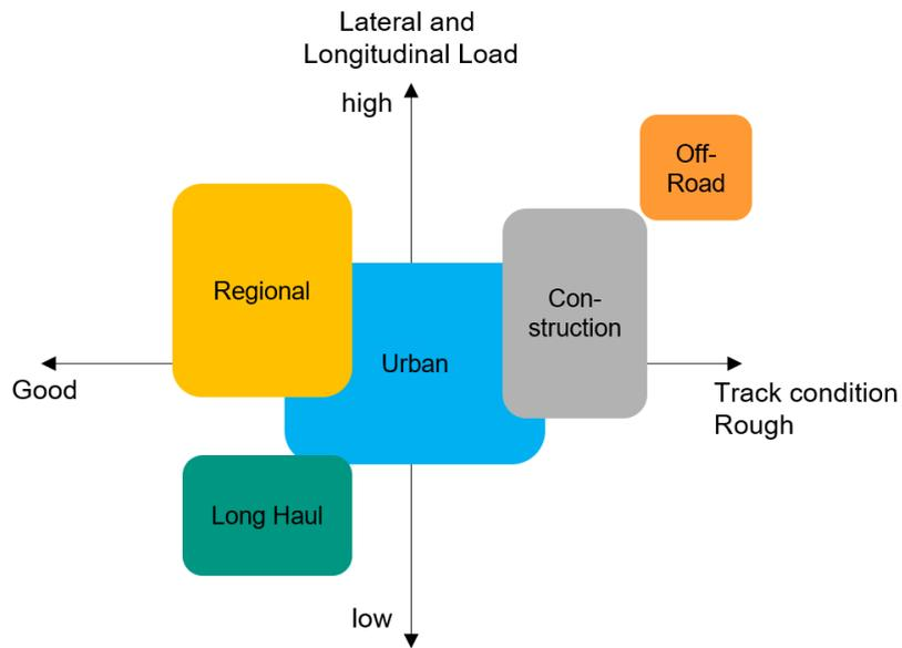
**Fig. 12.** Tires for commercial vehicle: Application oriented classification with special requirements on transmittable lateral and longitudinal forces and track condition, according to [9].
