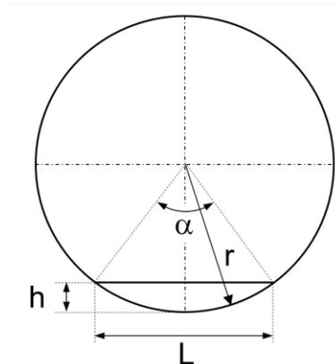
**Fig. 10.** Contact length  $L$  lead to curved contact with max. height of  $h$ .
