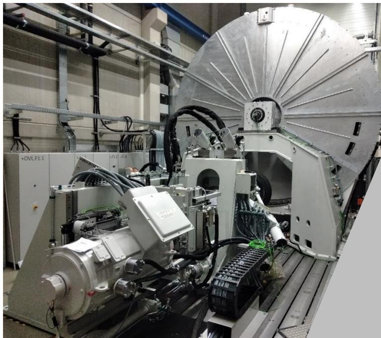
**Fig. 8.** New inner drum tire test bench GRIPS: Wheel drive and drum with cover.
