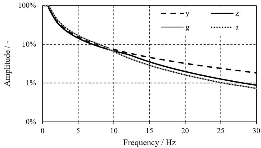
**Fig. 14.** Calculated target performance for movement of loaded wheel actuated by Hexapod: Maximum amplitude as frequency response for relevant actuation directions - Change of wheel position lateral (y) and vertical (z) and change of wheel camber angle (g) and slip angle (a) (100%:  $\Delta y = 115$  mm;  $\Delta z = 175$  mm;  $\Delta a = 18^\circ$ ;  $\Delta g = 18^\circ$ ); Source of calculated data: Inova GmbH
