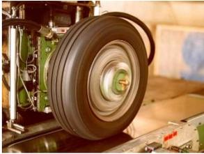
**Fig. 1** Tire rolling on flat track (steel band)
