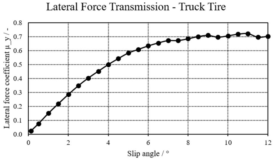
**Fig. 11.** Lateral force transmission - Truck tire: 445/50 R22.5;
