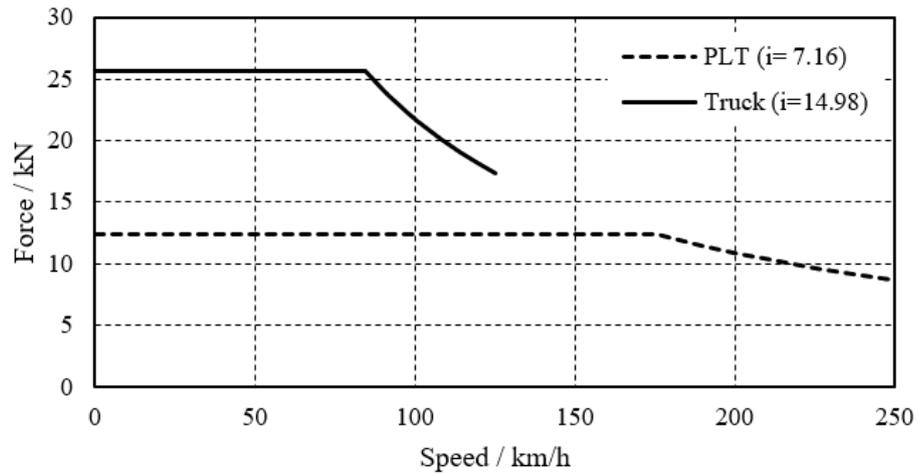
**Fig. 9.** Maximum longitudinal force delivered by drum drive (efficiency 95.7%) for the two selectable gear ratios.
