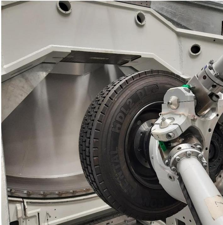
**Fig. 16.** Truck wheel mounted on the hexapod in front of the inner drum.
