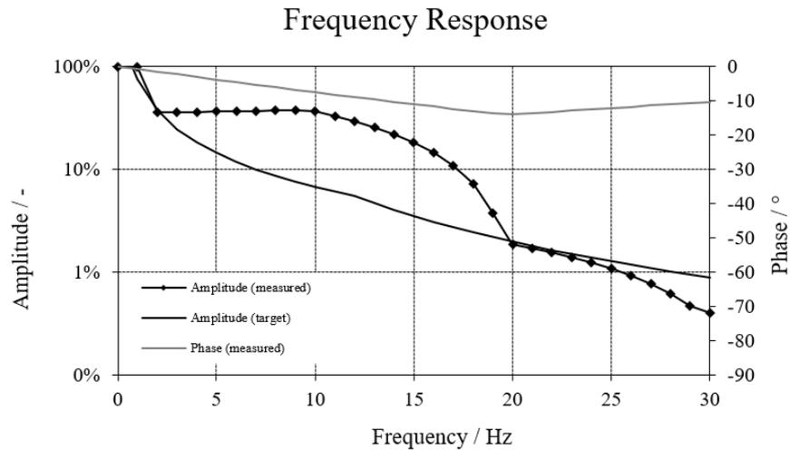
**Fig. 15.** Measured performance for movement of an unloaded wheel actuated by Hexapod: Maximum amplitude in z direction and phase shift as frequency response (100% amplitude:  $\Delta z = 175$  mm).
