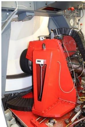
**Fig. 3.** Inner drum tire test bench with tire rolling inside a drum
