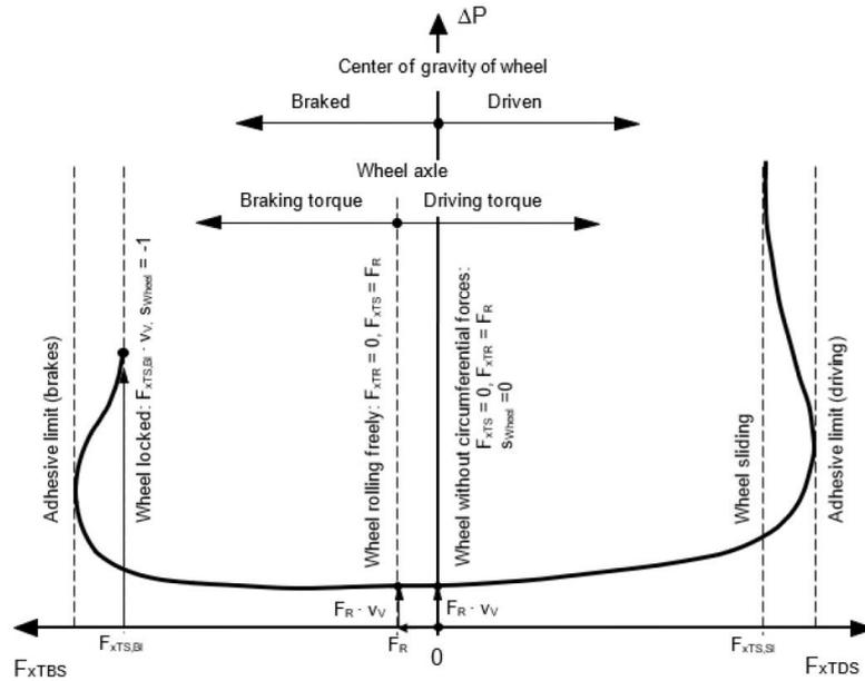
**Fig. 13.** Power loss  $\Delta P$  under constant vertical load, plotted against the circumferential force  $F_{xTS}$ , which is supported on the road as tractive force and can be measured as reaction force at the measuring wheel hub, translated from [13].
