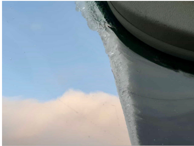
Figure 2.1: Ice accretion on the leading edge of a lightweight aircraft's airfoil. Minor incidents of runback icing are also indicated (Photo taken during private flight by a hobby pilot).
