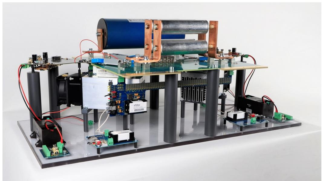
**Figure 8.** The double power electronic building block for the flying capacitor converter.
