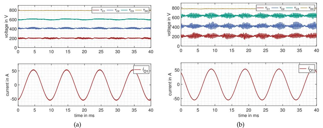
**Figure 15.** Single phase capacitor voltage, output voltage, and output current waveforms with the same output current and DC-link voltage set point. (a) Measurements results of the first method [4] balancing algorithm—fixed switching sequences and variable plateau time  $t_p$ . (b) Measurements results of the second method [2] balancing algorithm—variable switching sequences and fixed plateau time  $t_p$ .
