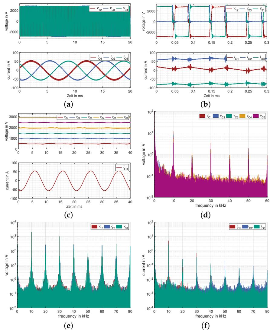
**Figure 17.** Measurement results at medium voltage with  $V_{DC} = 2.9$  kV and 100 Hz output frequency. (a) Three-phase output voltage and output current waveforms. (b) Three-phase output voltage and output current waveforms. (c) Single-phase output current and capacitor voltages waveforms. (d) Frequency spectrum of the capacitor voltage waveforms. (e) Frequency spectrum of the output voltage waveforms. (f) Frequency spectrum of the output current waveforms.
