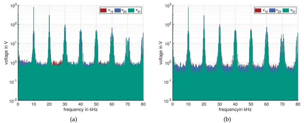
**Figure 12.** Three-phase output voltage frequency spectrum with the same output current and DC-link voltage set point. (a) Measurements results of the first method [4] balancing algorithm—fixed switching sequences and variable plateau time  $t_p$ . (b) Measurements results of the second method [2] balancing algorithm—variable switching sequences and fixed plateau time  $t_p$ .
