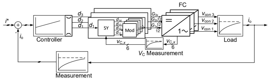
Figure 4. Signal structure of Q2O of FCC.
