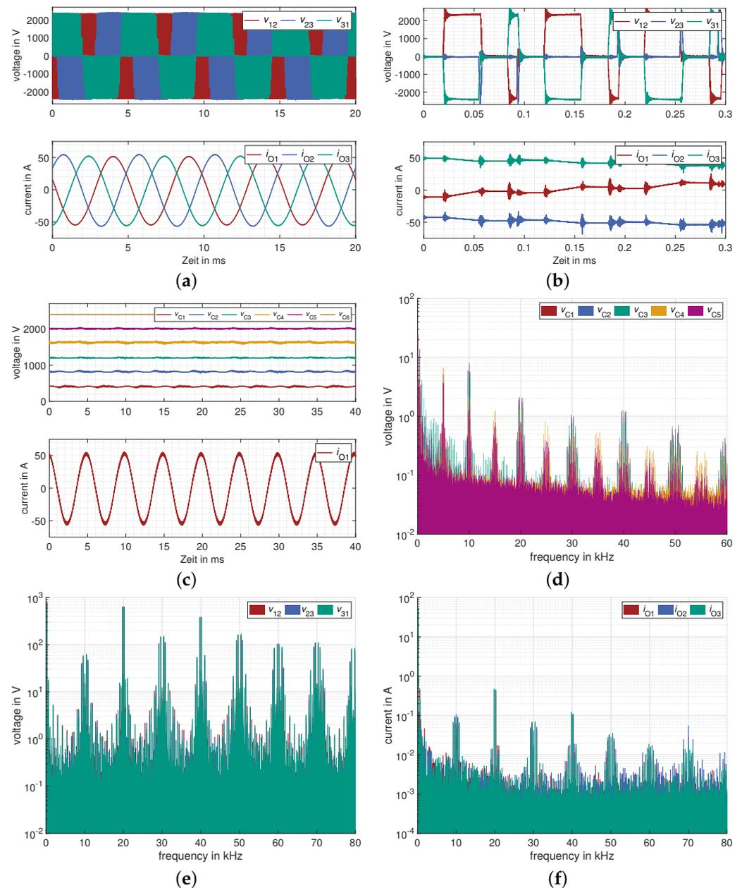
**Figure 18.** Measurement results at medium voltage with  $V_{DC} = 2.4$  kV and 200 Hz output frequency. (a) Three-phase output voltage and output current waveforms. (b) Three-phase output voltage and output current waveforms. (c) Single-phase output current and capacitor voltages waveforms. (d) Frequency spectrum of the capacitor voltage waveforms. (e) Frequency spectrum of the output voltage waveforms. (f) Frequency spectrum of the output current waveforms.
