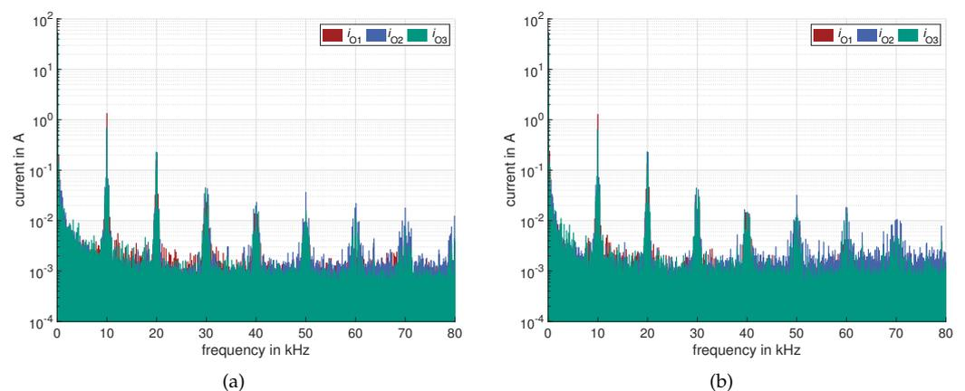
**Figure 13.** Three-phase output current frequency spectrum with the same output current and DC-link voltage set point. (a) Measurements results of the first method [4] balancing algorithm—fixed switching sequences and variable plateau time  $t_p$ . (b) Measurements results of the second method [2] balancing algorithm—variable switching sequences and fixed plateau time  $t_p$ .
