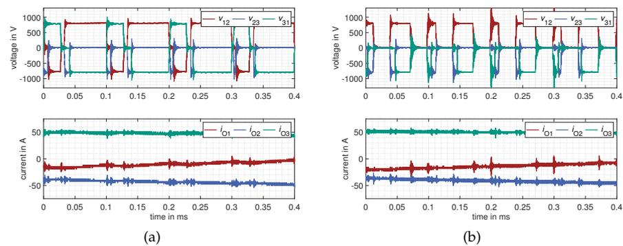
**Figure 14.** Three-phase output voltage and output current waveforms with the same output current and DC-link voltage set point. (a) Measurements results of the first method [4] balancing algorithm—fixed switching sequences and variable plateau time  $t_p$ . (b) Measurements results of the second method [2] balancing algorithm—variable switching sequences and fixed plateau time  $t_p$ .
