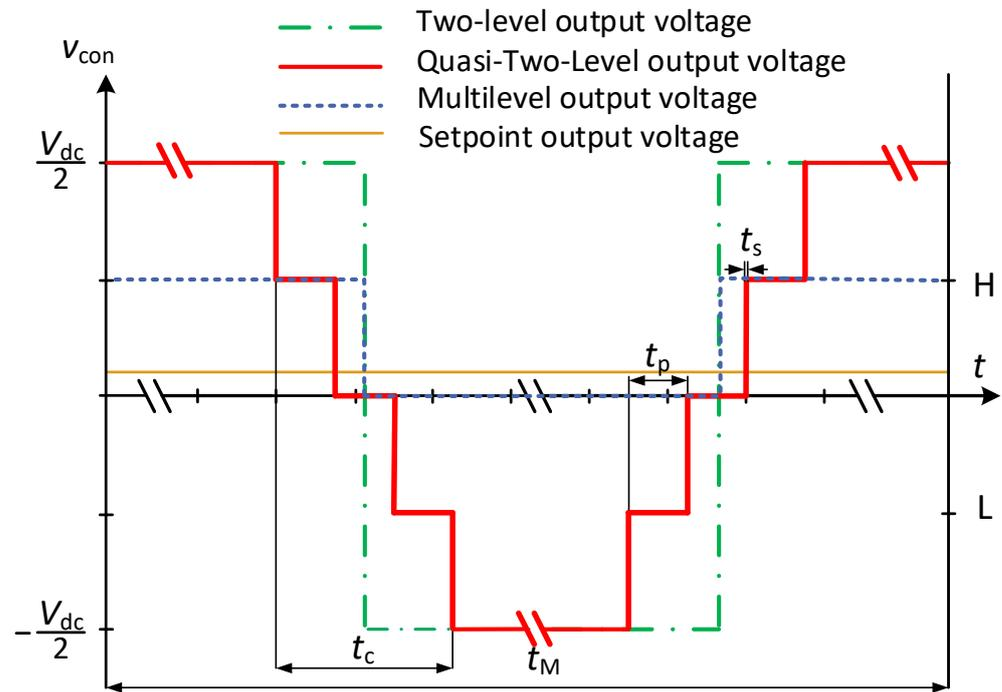
**Figure 3.** Quasi-Two-Level output voltage principle.
