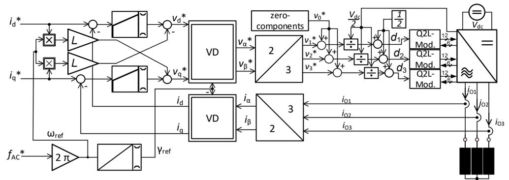
Figure 5. Signal structure of the output current controller.
