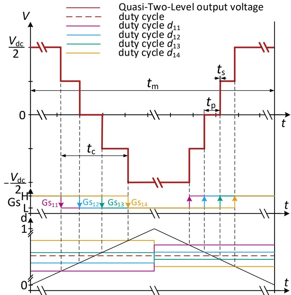
Figure 7. Carrier-based modulation with the balancing of the Q2O at FCC.
