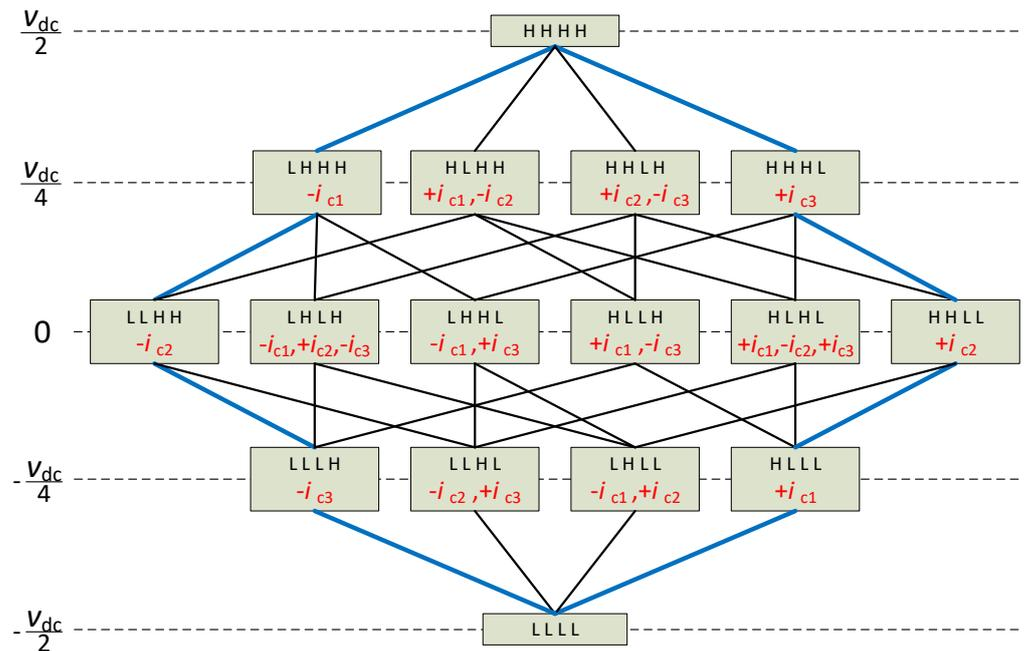
**Figure 6.** Switching state chart for a 5-level flying capacitor.
