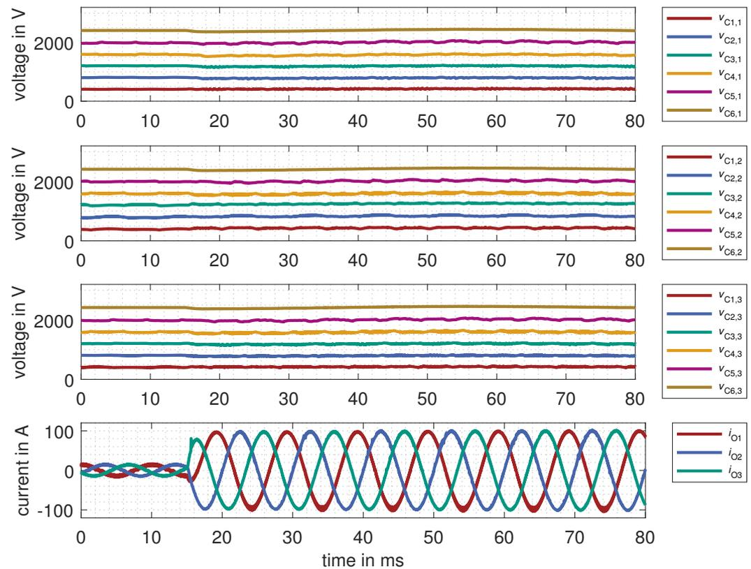
**Figure 20.** Output current set point step measurement results at medium voltage with  $V_{DC} = 2.4$  kV.
