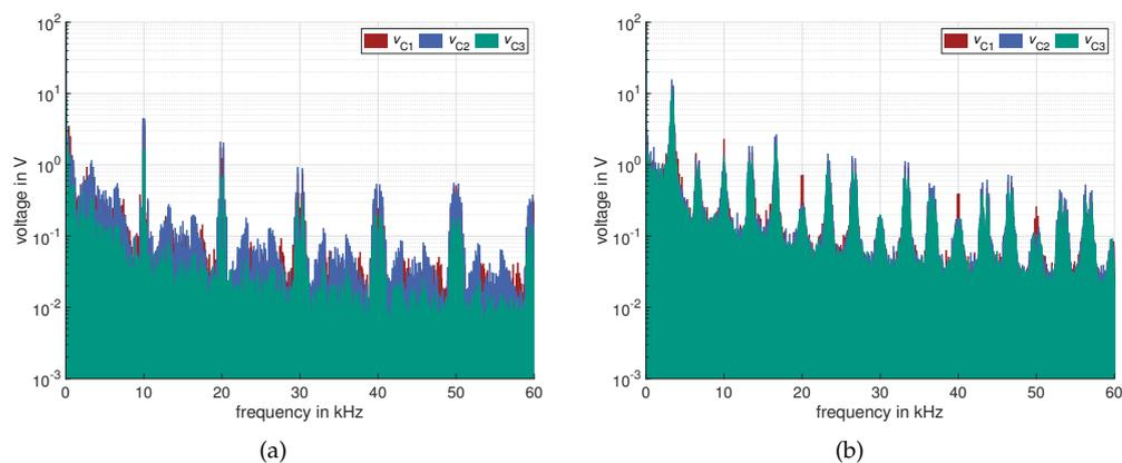
**Figure 16.** Single phase frequency spectrum of the capacitor voltage waveforms with the same output current and DC-link voltage set point. (a) Measurements results of the first method [4] balancing algorithm—fixed switching sequences and variable plateau time  $t_p$ . (b) Measurements results of the second method [2] balancing algorithm—variable switching sequences and fixed plateau time  $t_p$ .
