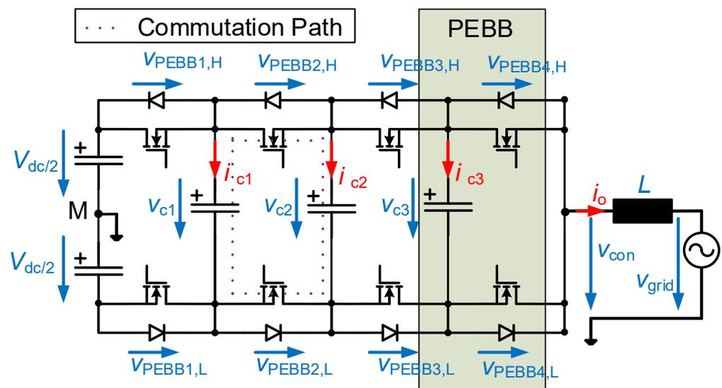
**Figure 1.** One phase leg of a five-level flying capacitor converter.
