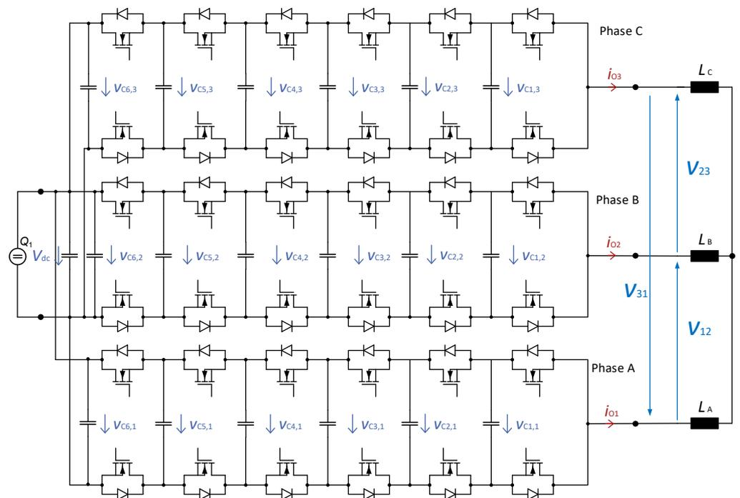
Figure 10. Three-phase test-setup.
