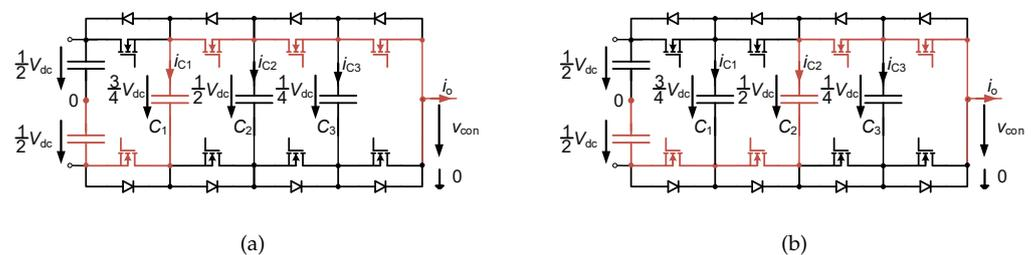
**Figure 2.** Exemplary switching states of the FCC. (a) State *LHHH* with  $+\frac{V_{dc}}{4}$  output voltage. (b) State *LLHH* with zero output voltage.
