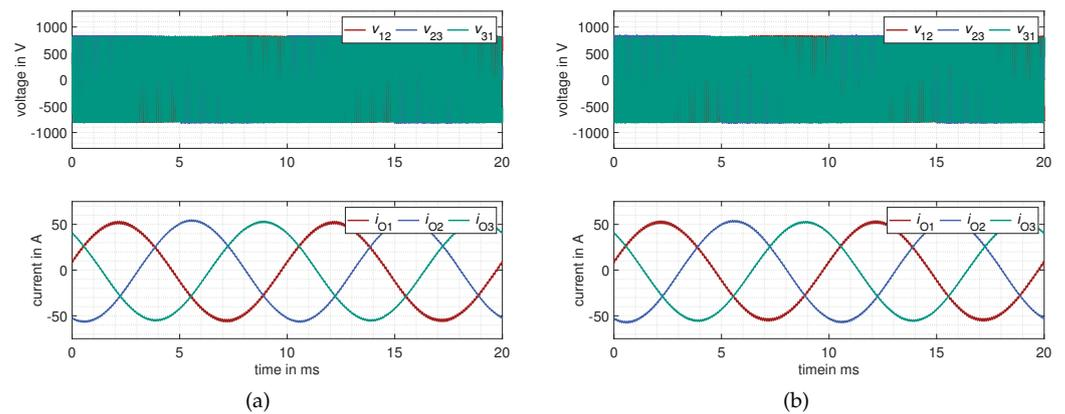
**Figure 11.** Three-phase output voltage and output current waveforms with the same output current and DC-link voltage set point. (a) Measurements results of the first method [4] balancing algorithm—fixed switching sequences and variable plateau time  $t_p$ . (b) Measurements results of the second method [2] balancing algorithm—variable switching sequences and fixed plateau time  $t_p$ .
