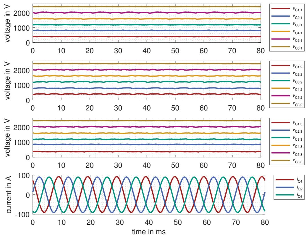
**Figure 19.** Steady-state measurement results at medium voltage with  $V_{DC} = 2.4$  kV and 100 A.
