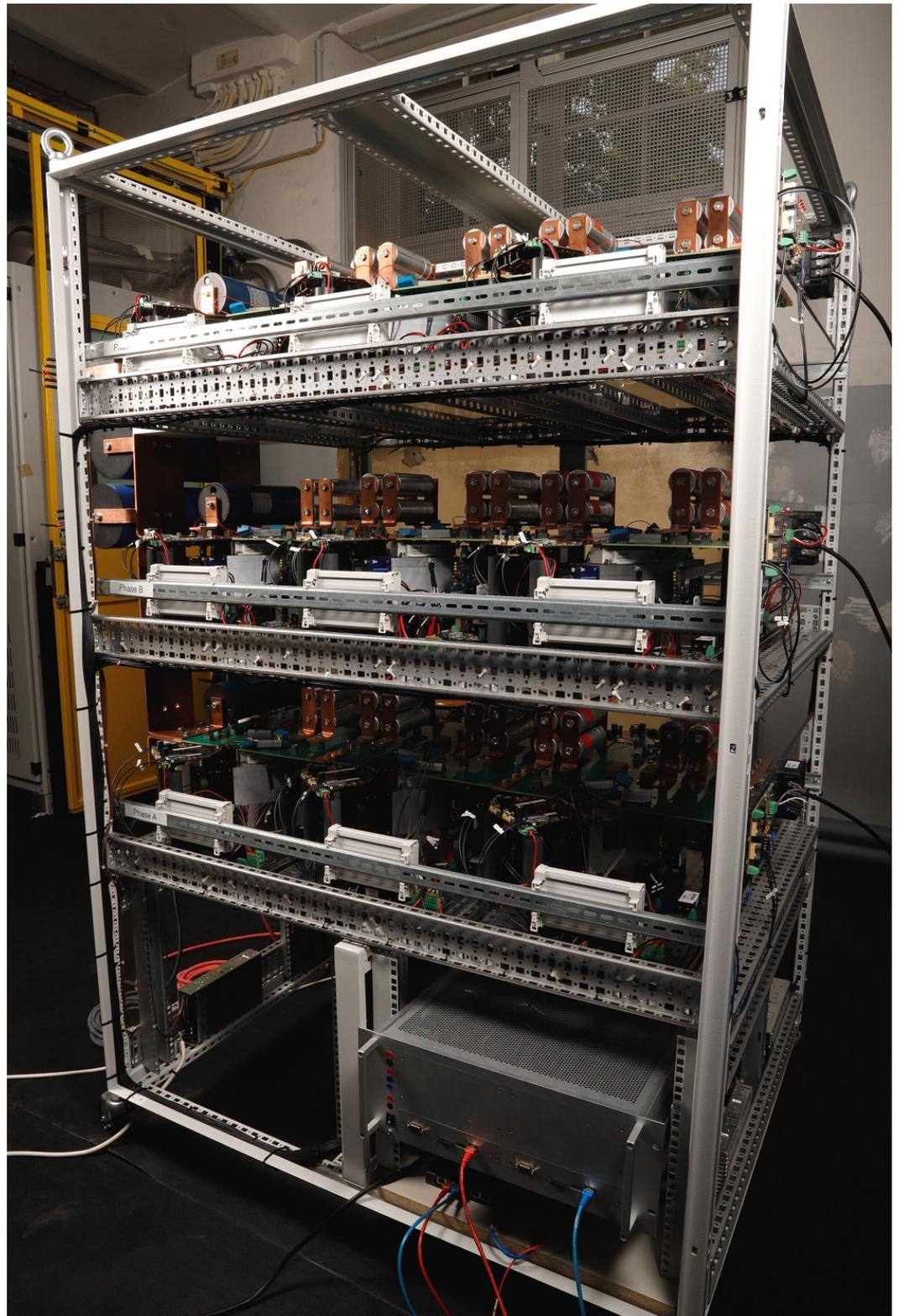
**Figure 9.** Picture of the three-phase seven-level flying capacitor converter.
