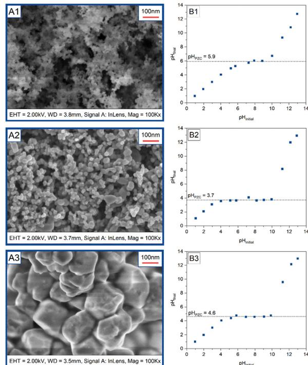
Fig. 1 SEM images of support materials (A1: SiO<sub>2</sub>, A2: TiO<sub>2</sub>, A3: ZrO<sub>2</sub>) and final pH value as function of initial pH value (B1: SiO<sub>2</sub>, B2: TiO<sub>2</sub>, B3: ZrO<sub>2</sub>) in PZC determination.
