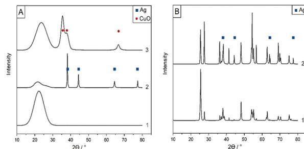
Fig. 7 XRD patterns of Ag and Cu catalysts after the catalytic reaction (after 7 h TOS at 575 °C). Silica supported catalysts (A: SiO<sub>2</sub> (1), Ag/SiO<sub>2</sub> 3 × 500 m<sup>2</sup> L<sup>-1</sup> (2), Cu/SiO<sub>2</sub> 3 × 500 m<sup>2</sup> L<sup>-1</sup> (3)); titania-supported catalyst (B: TiO<sub>2</sub> (P25) (1), Ag/TiO<sub>2</sub> 2 × 500 m<sup>2</sup> L<sup>-1</sup> (2)).
