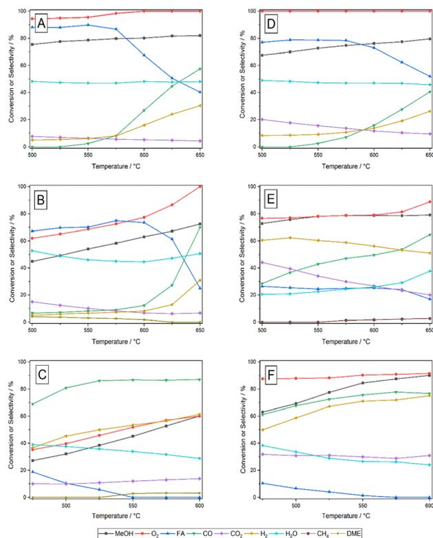
**Fig. 3** Conversion and selectivity as function of temperature for Ag/SiO<sub>2</sub> (A), Ag/TiO<sub>2</sub> (B), Ag/ZrO<sub>2</sub> (C), Cu/SiO<sub>2</sub> (D), Cu/TiO<sub>2</sub> (E) and Cu/ZrO<sub>2</sub> (F) with CSA = 1000 m<sup>2</sup> L<sup>-1</sup> in all cases. Feed: 2.5% methanol and 1.0% oxygen in nitrogen, total flow rate: 1 L<sub>STP</sub> min<sup>-1</sup>, TOS: 8 h.
