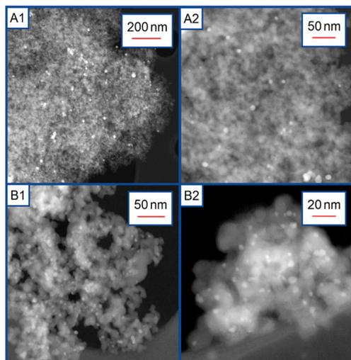
Fig. 6 STEM-HAADF images of the catalysts after catalytic reaction (A1 and A2: Ag/SiO<sub>2</sub> 1000 m<sup>2</sup> L<sup>-1</sup>, B1 and B2: Cu/SiO<sub>2</sub> 1000 m<sup>2</sup> L<sup>-1</sup>).
