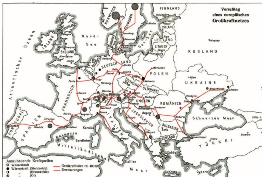
Figure 1: First European Electricity System Network Plan, as suggested by Oskar Oliven in 1930 [9].
