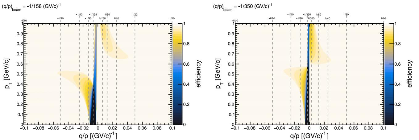
FIG. 19. Efficiency of the interaction trigger for particles with a certain curvature  $q/p$  and transverse momentum  $p_T$  for the two beam energies 158 (left, trigger radius 0.9 cm) and 350 GeV/c (right, trigger radius 0.6 cm).
