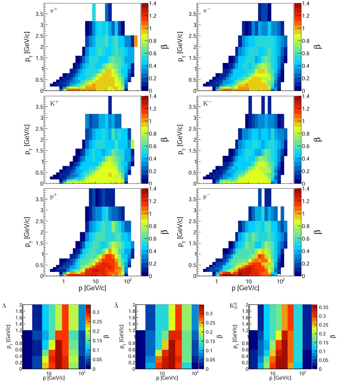
FIG. 8.  $\beta$  correction factors for the 158 GeV/c dataset (see Fig. 23 in the Appendix C for  $p_{\text{beam}} = 350$  GeV/c).
