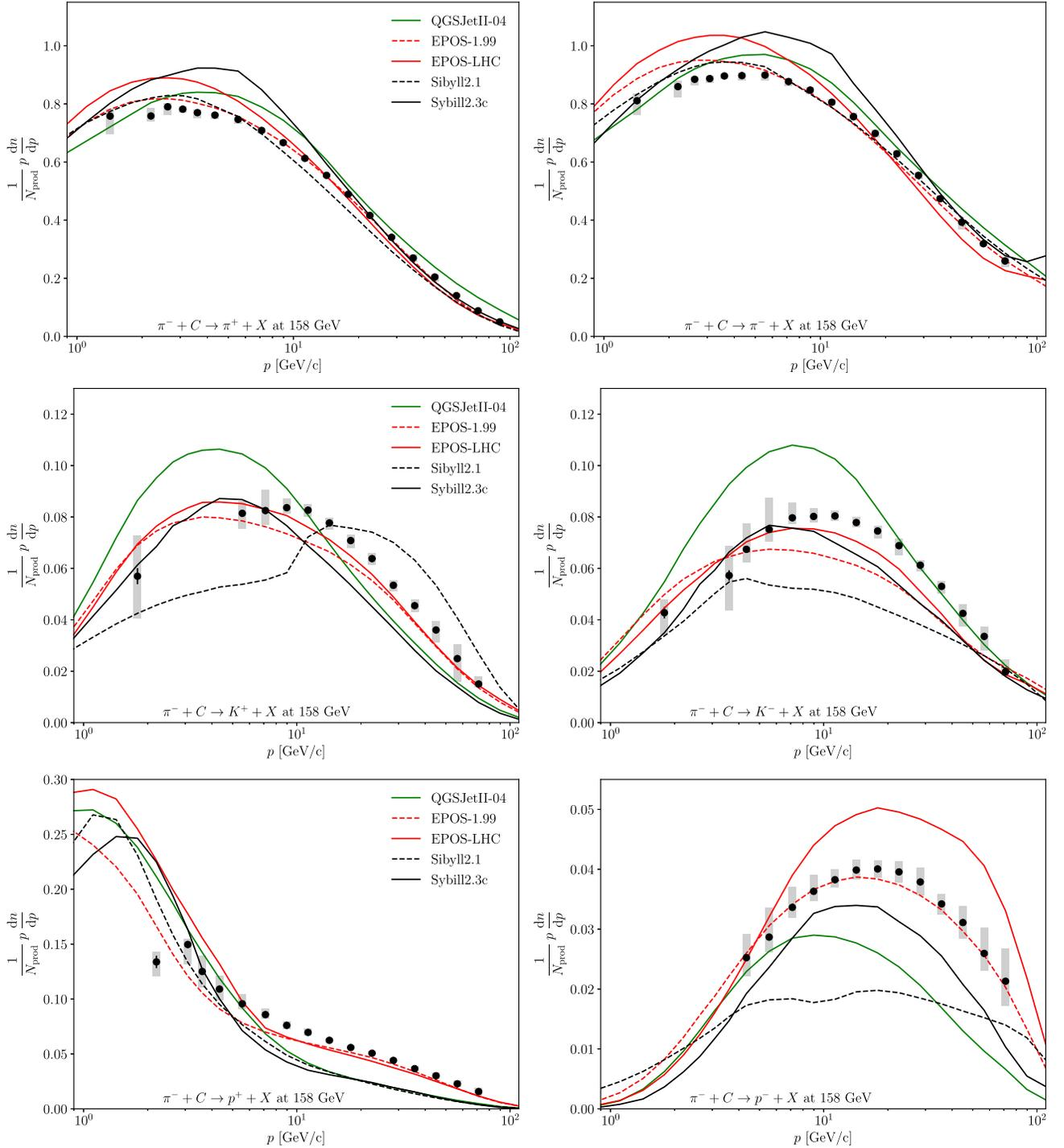
FIG. 15. Comparison of the  $p_T$ -integrated particle production spectra of  $\pi^\pm$ ,  $K^\pm$ , and  $p(\bar{p})$  at 158 GeV/ $c$  with predictions of hadronic interaction models. The data is shown as black circles with statistical error bars. Systematic uncertainties are displayed by gray rectangles.
