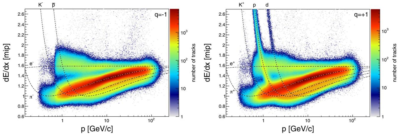
FIG. 25. Energy deposit vs momentum of negatively and positively charged tracks for the 350 GeV/c dataset. The dashed lines indicate the average energy deposit for each particle type.
