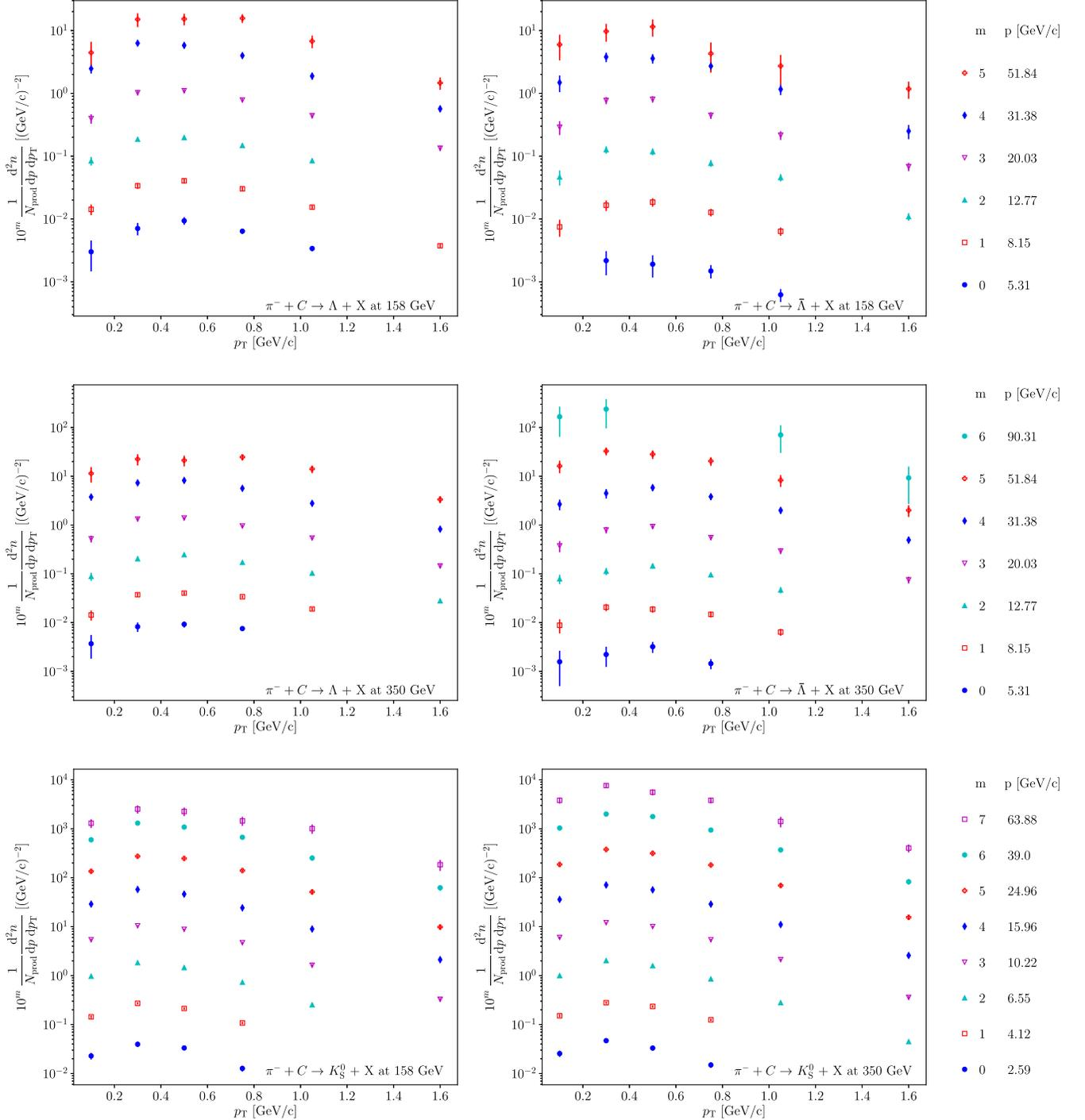
FIG. 13. Production spectra of  $\Lambda$ ,  $\bar{\Lambda}$ , and  $K_S^0$  in  $\pi^-$ -C interactions at  $p_{\text{beam}} = 158$  and  $350$  GeV/c. For each bin in momentum  $p$ , the spectrum was multiplied by  $10^m$  with the value of  $m$  shown on the right. Error bars show the statistical uncertainties.
