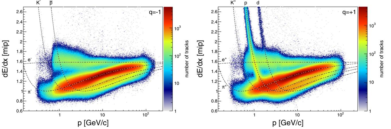
FIG. 6. Energy deposit vs momentum of negatively and positively charged tracks for the 158 GeV/c dataset. The dashed lines indicate the average energy deposit for each particle type (see Fig. 25 in the Appendix C for  $p_{\text{beam}} = 350$  GeV/c).
