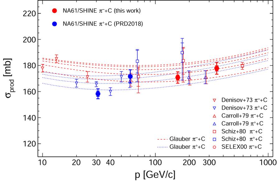
FIG. 4. Production cross section in  $\pi^-$ -C interactions (red) and  $\pi^+$ -C interactions (blue). Measurements by NA61/SHINE are shown as filled circles, previous measurements from [58,61–63] are indicated by open symbols. Predictions from the Glauber model with different values of the inelastic screening are shown as dashed lines ( $\lambda = 0.1, 0.3, 0.5, 0.7,$  and  $0.9$  from top to bottom).
