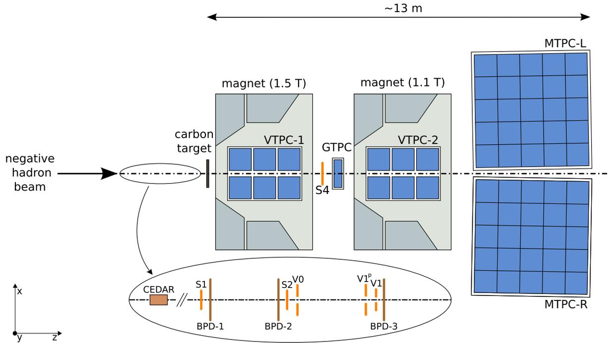
FIG. 2. Experimental setup of the NA61/SHINE experiment [25] (configuration for the  $\pi^-$ -C data taking). The coordinate system used in this paper is indicated on the lower left. The incoming beam direction is along the  $z$  axis. The magnetic field bends charged particle trajectories in the  $x-z$  (horizontal) plane. The drift direction in the TPCs is along the  $y$  (vertical) axis. A zoomed view of the beam and trigger instrumentation is shown as an elliptical inset at the bottom.
