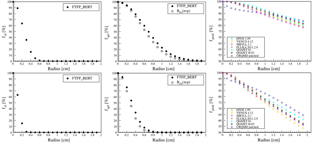
FIG. 20. Fraction of events leading to a forward particle within a given radial trigger distance from the beam. Columns show from left to right simulations of elastic, quasielastic, and production interactions. The top row shows the fractions for beam energies of 158 GeV/c and the bottom row for 350 GeV/c.
