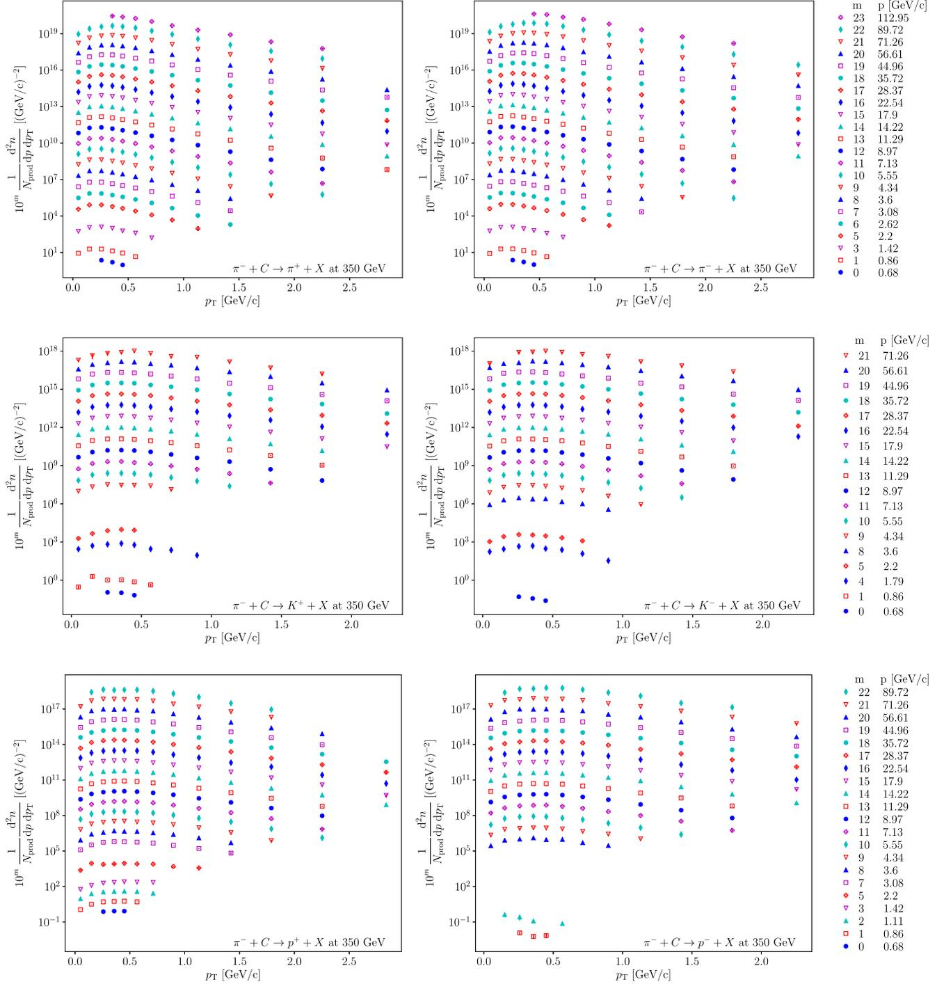
FIG. 12. Production spectra of  $\pi^\pm$ ,  $K^\pm$ , and  $p(\bar{p})$  in  $\pi^-$ -C interactions at  $p_{\text{beam}} = 350$  GeV/c. For each bin in momentum  $p$ , the spectrum was multiplied by  $10^m$  with the value of  $m$  shown on the right. Error bars show the statistical uncertainties and are most of the times smaller than the marker size.
