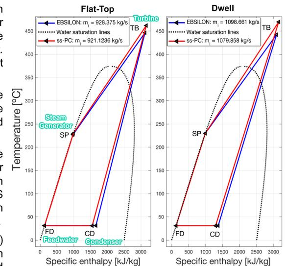
Figure 3: Simplified thermodynamical cycle diagrams for the Power Conversion System (PCS) Subcycle, with points indicating mass-averaged inlet values of properties for heat transfer fluid (water). Connecting lines are only representative: evaporation has fixed temperature in steam generator and turbine presents multiple outlets, both taken into account by the model.
