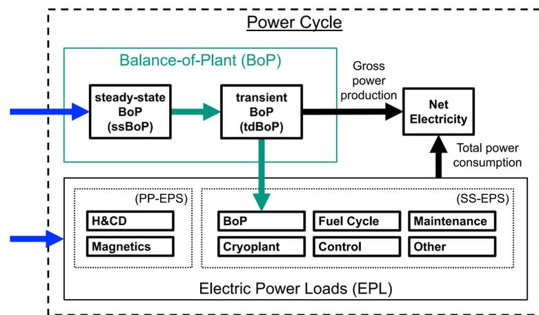
Figure 1: Data transfer in Power Cycle module architecture. Initial characterization depends on assumptions and design parameters (blue arrows). Main results of the BoP sub-module are presented in this work (green arrows). The final output foreseen is a time-dependent curve of the net electrical power generated, computed from gross production and total consumption (black arrows).
