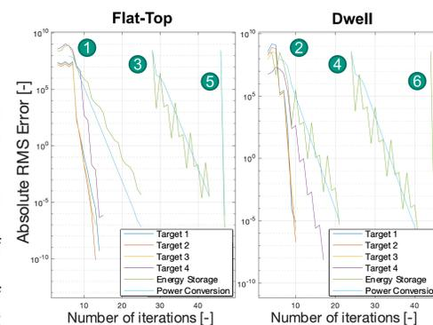
Figure 2: Visualization of the multi-tiered iterative computation of the BoP model, until total absolute RMS error is below a certain threshold. Each curve shows the error reduction from updating a single Subcycle; error reduction is non-monotonic because of Coupling between Subcycles in a single phase. Coupling between phases implies each phase must be updated multiple times (green numbers indicate order of update).
