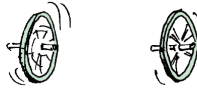
Fig. 3.12 The wheel that rotates fast has more angular momentum than the wheel that rotates slowly.
