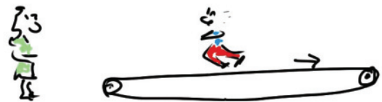
Fig. 10.4 Willy will only reach Lilly if he moves to the left faster than the moving walkway moves to the right.
