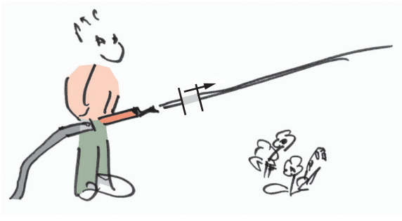
Fig. 2.38 The momentum of a water portion moves with the water portion: convective momentum current.
