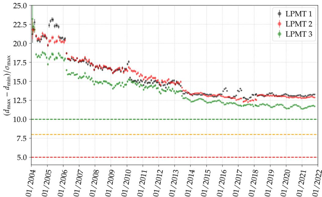
**Figure 6.25:** Monthly averages of relative density differences of the muon maximum and its accompanying minimum for the three LPMTs of the station LS324. The green, orange, and red horizontal dashed lines highlight threshold factors for the search condition of the limits around the extreme values with  $f = 10, 8, 5$ .
