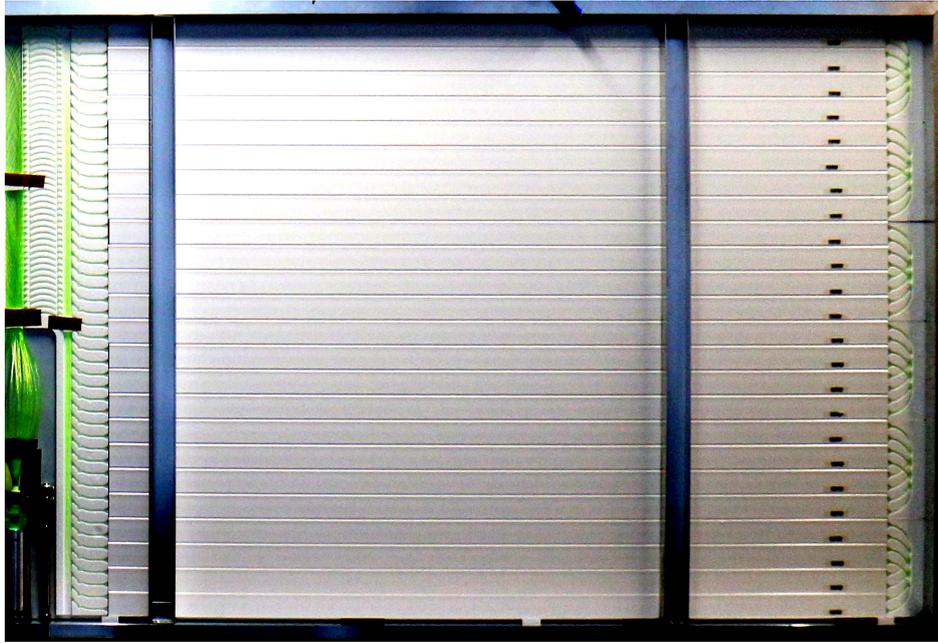
**Figure 3.12:** Top view of a completed wing of an [SSD](#), including the 24 narrowly arranged scintillator bars, the [WLS](#) fibers inserted in the bars and routed by the [XPS](#) forms towards the readout device. Taken from Ref. [108].
