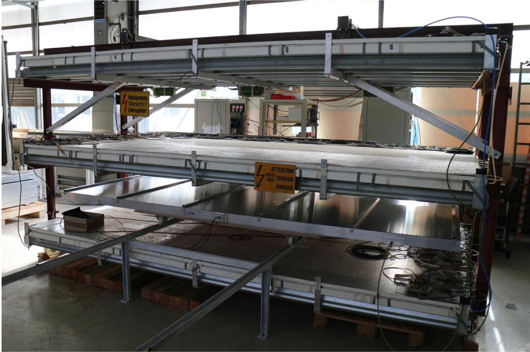
**Figure 4.1:** Photo of the muon tower during the SSD validation tests. The set-up shows the three planes of LST chambers. An SSD is inserted between the center and the bottom plane on top of the movable support structure.
