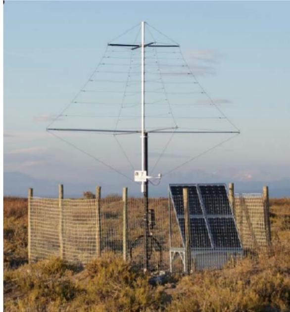
**Figure 3.9:** Photo of a ratio antenna of the type LPDA installed in the AERA. The antenna, receiver, and electronics are powered by a solar panel. Taken from Ref. [86].
