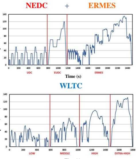
$\succ$  Chassis dynamometer tests in a test cell (T = 23 ± 3 °C; RH = 50 ± 5 %) > Tests with NEDC, WLTC, and ERMES (hot start) driving cycle
