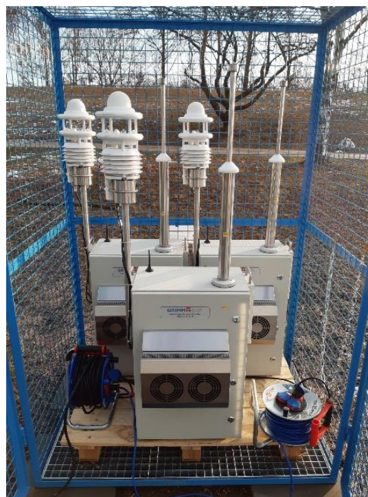
All three CPCs in the grid box. Left: at the place of the aerosol-measurement station in Augsburg | Right: next to the UFP measurement station of the Bavarian State Agency for Environment (University of Regensburg)
