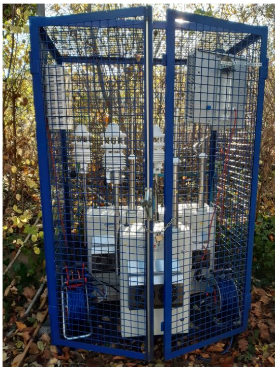
All three CPCs in the grid box. Left: at the place of the aerosol-measurement station in Augsburg | Right: next to the UFP measurement station of the Bavarian State Agency for Environment (University of Regensburg)
