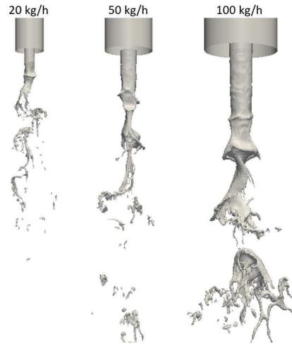
FIG. 5. Iso-surfaces of calculated liquid volume fraction at  $f = 0.5$  for up-scaled nozzles.
