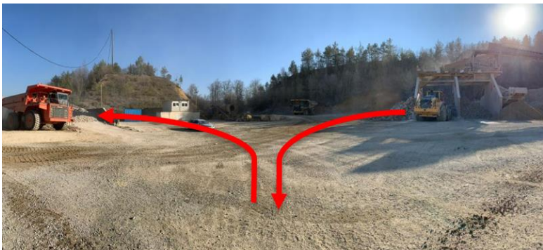
Figure 4.12: Wheel-loader transfers sized materials
