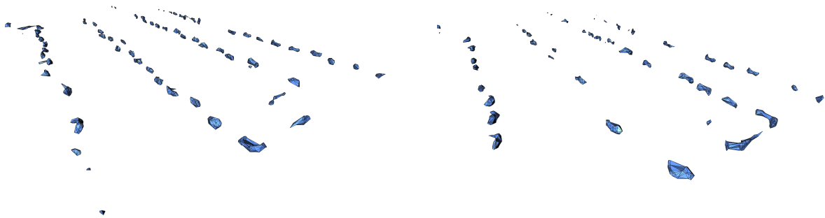
Figure 6.27: Illustration of an exemplary surface reconstruction of the isolated vehicle detections in a car park from two different semantic radar SLAM maps. The bumper shells are prominently reconstructable for the passed vehicle rows.
