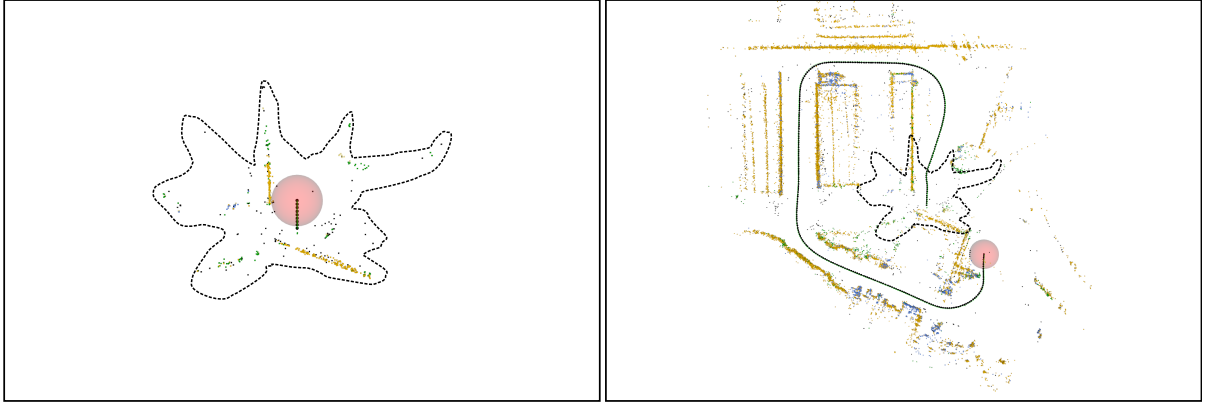
Figure A.11: Illustration of the automated initialization drive resulting semantic radar SLAM map (left), with respect to the reference map (right) of the test scenario B. The sub-sampled and convex-hull extract is depicted as dashed line.
