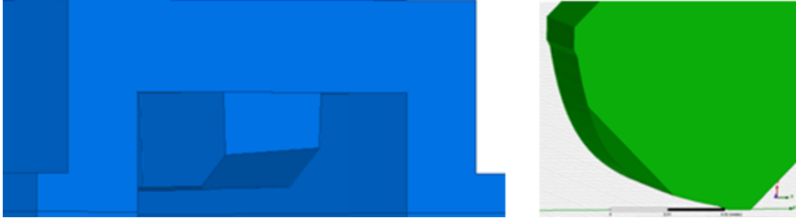
Figure 2.20.: Chamfers on H-type dipole magnet (left) and quadrupole magnets (right).
