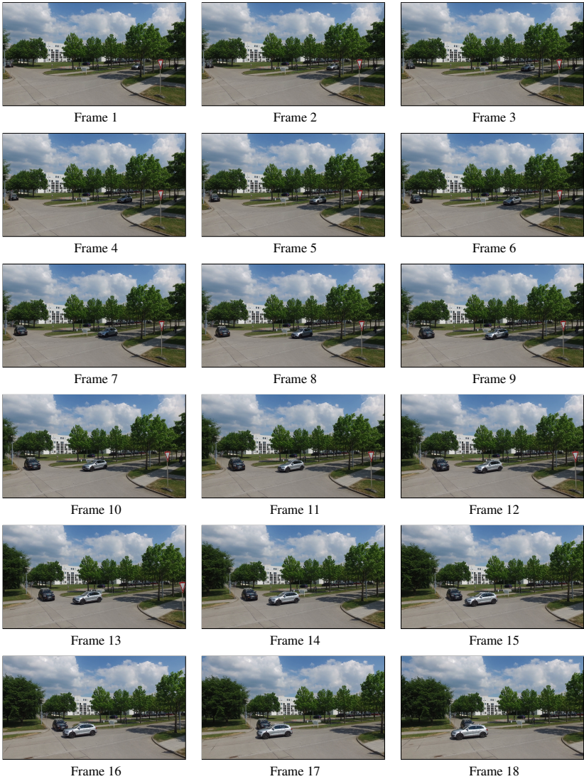
Figure 7.4: Safe intersection crossing in the presence of noncompliant participants. The autonomous vehicle (gray) has the right of way. The speed of the oncoming black vehicle suggests that it will not yield to gray vehicle. Frames are incremented every 0.25 s.
