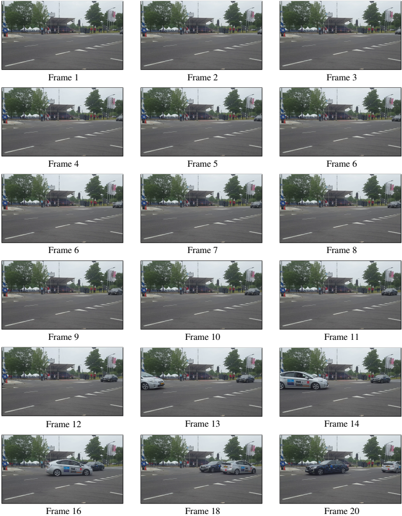
Figure 7.2: Cooperative intersection crossing. 1 Frames are incremented every 0.25 s. Later frames, in which the vehicle ID 150 is visible, are omitted.
