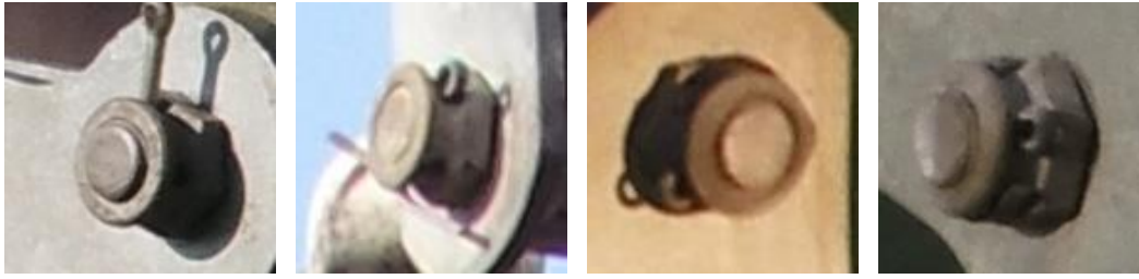
Fig. 6.4.: Exemplary images of the safetypin component type from the DS3_{Pi} dataset. The defective safetypins (two to the left) are not completely bent, while the intact ones (two to the right) are completely bent and consequently prevent slipping out.
