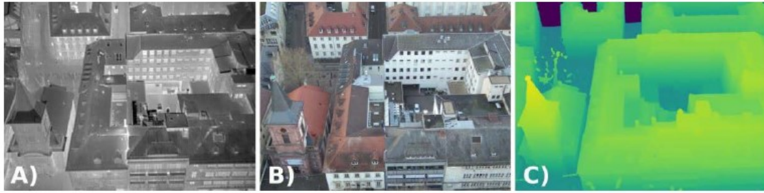
Figure 5: Drone images of the city center of Karlsruhe used for the TBBR dataset presented in Paper E: (A) thermal image, (B) RGB image, and (C) image with height information (Original source: Mayer et al., 2021 – Paper E)
