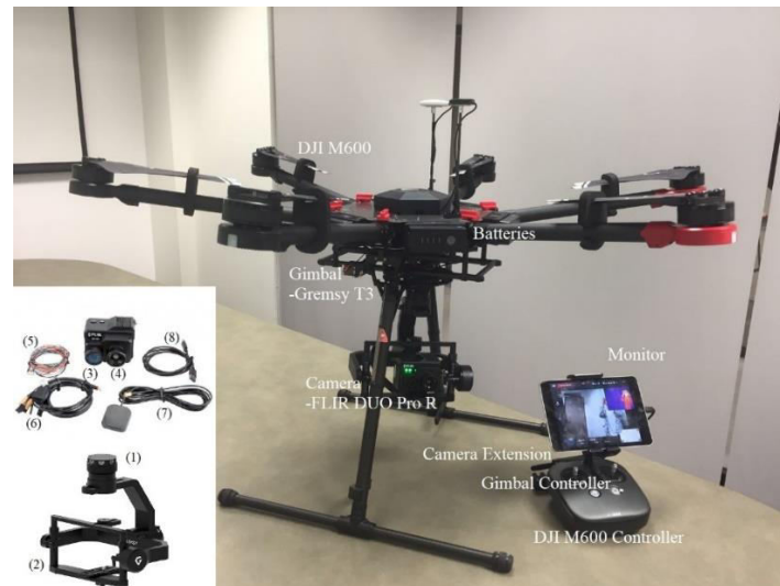
(1) Gimbal - Connection to DJI M600; (2) Gimbal - Frame for Camera; (3) FLIR DUO Pro R – Visible Lens Barrel; (4) FLIR DUO Pro R – IR Lens Barrel; (5) FLIR DUO Pro R – Electric Wires; (6) FLIR DUO Pro R – Integration Cable; (7) FLIR DUO Pro R – GPS Antenna Cable; (8) FLIR DUO Pro R – USB Cable.
